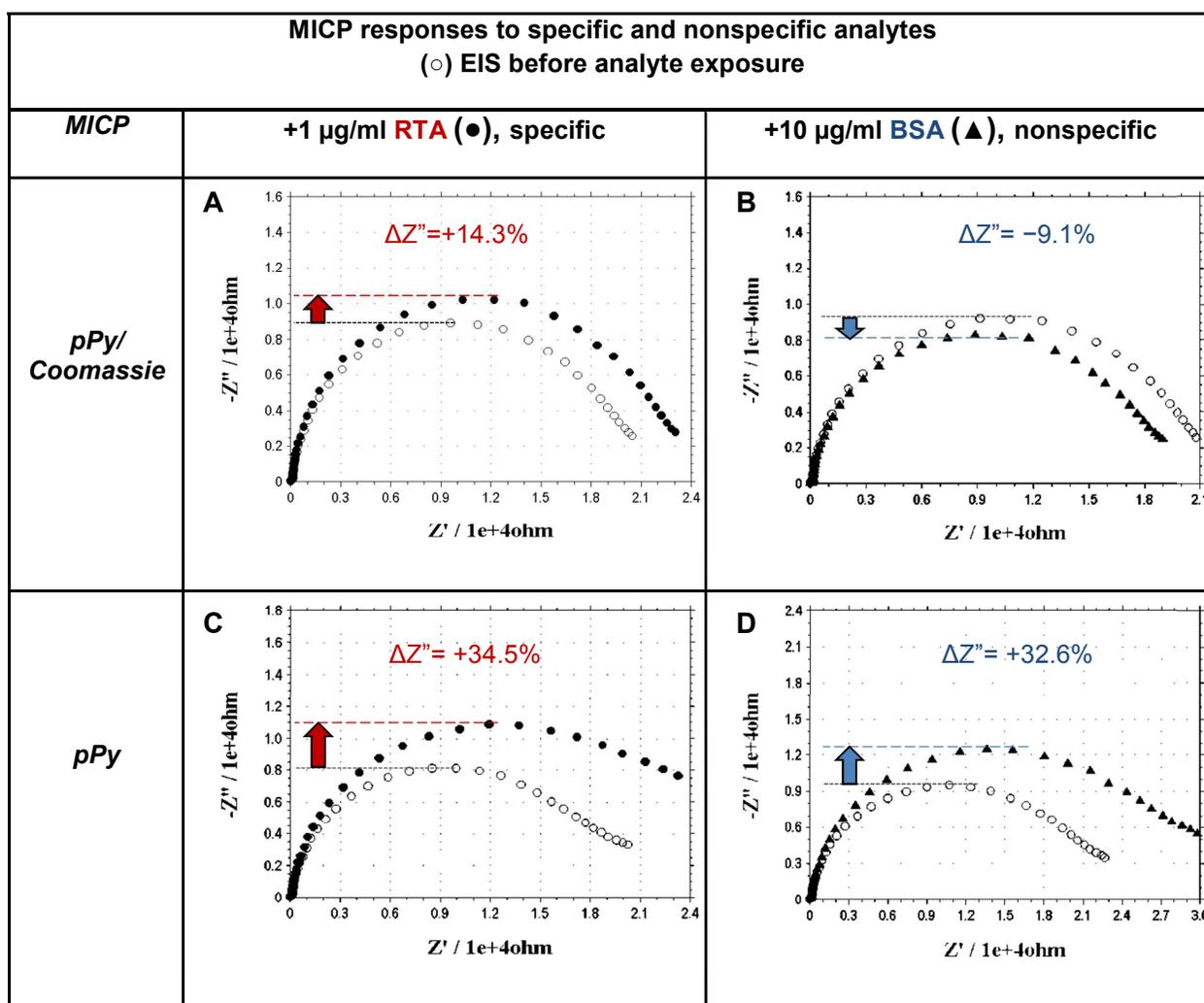
**Figure 3. Macromolecular dopant is needed for specificity of MICP.** Impedance changes in RTA-imprinted pPy/Coomassie MICP (A&B) and in pPy MICP (C&D) upon interaction with specific analyte (●): 1  $\mu\text{g/ml}$  RTA, A&C; and nonspecific analyte (▲): 10  $\mu\text{g/ml}$  BSA, B&D. (○): EIS spectra before incubation.
