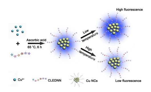
We have developed a simple and green method for synthesis of blue fluorescent peptide-templated Cu nanoclusters (NCs). The as-prepared Cu NCs display temperature dependent fluorescence and low toxicity, which can be employed as a fluorescent probe for temperature sensing and cellular imaging.
