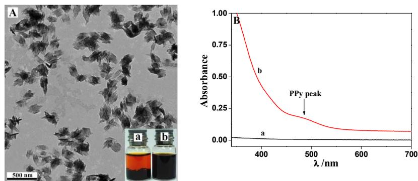
**Fig. 1.** Characterization of PPy-F127 NPs. (A) TEM image of the PPy-F127 NPs, inset: (bottle a) PPy in the absence of F127, and (bottle b) PPy-F127 NPs. (B) UV-*vis* adsorption spectra of (a) F127 aqueous solution, and (b) PPy-F127 NPs.
