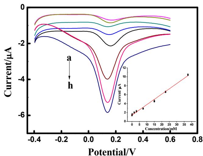
**Fig. 4.** DPVs obtained at Nafion/LOx/(PPy-F127)/GCE in 0.1 M PBS (pH=7.4) with the concentration of L-lactic acid (from a to h) 0.015, 0.15, 1.5, 3, 7.5, 15, 22.5, 37.5 mM. The parameters were as follows: pulse amplitude of 50 mV, pulse width of 50 ms and voltage range from -0.4 to 0.6 V. The insert: calibration curve for L-lactic acid obtained at the Nafion/LOx/(PPy-F127)/GCE biosensor.
