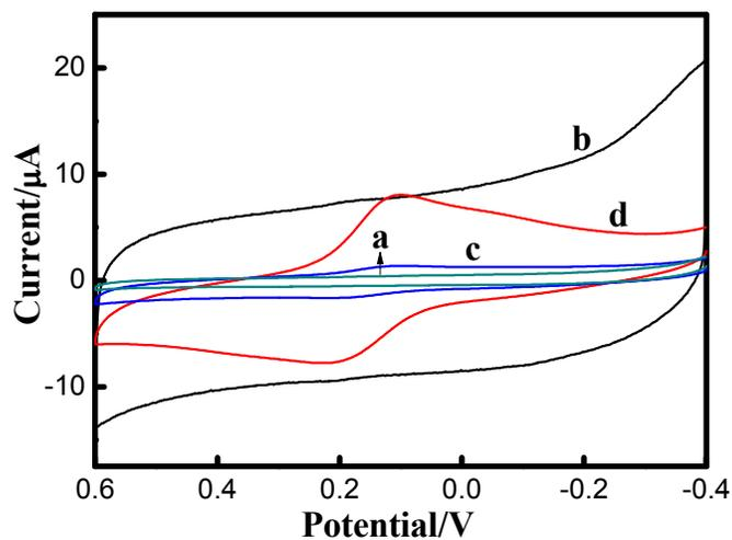
**Fig. 3.** CVs of (a) bare electrode, (b) PPy-F127 NPs film modified electrode, (c) Nafion/LOx/(PPy-F127)/GCE in 0.1 M PBS (pH=7.4), and (d) Nafion/LOx/(PPy-F127)/GCE in 0.1 M PBS (pH=7.4) with the concentration of L-lactic acid 10 mM. Scan rate: 100 mV/s.
