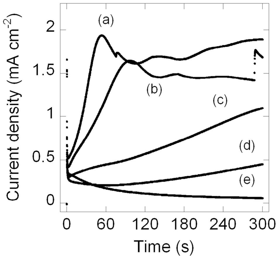
Figure 3. Variations of reduction currents on GC electrodes in 0.1 M phosphate buffer containing Pt complexes at -1.1 V. Concentrations of complexes are (a) 10, (b) 5.0, (c) 2.5, (d) 0.5 and (e) 0  $\mu\text{M}$ .
