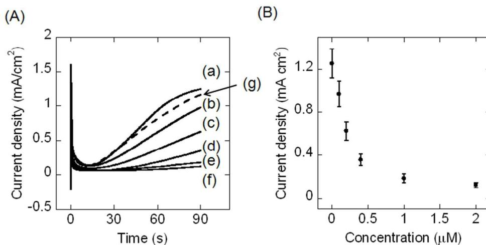
(A) Current-time curves in 0.1 M phosphate buffer containing 5.0 μM Pt complex, 1.0 μM capture DNA and the different concentrations of target DNA. Concentrations of target DNA: (a) 0, (b) 0.1, (c) 0.2, (d) 0.4, (e) 1.0 and (f) 2.0 μM. (g) Response obtained in the presence of 1.0 μM ssDNA with a non-complementary sequence to the capture DNA. (B) Relationship between the target DNA concentration and the reduction currents obtained 90 s after applying the potential.  $\mu$  66x34mm (300 x 300 DPI)
