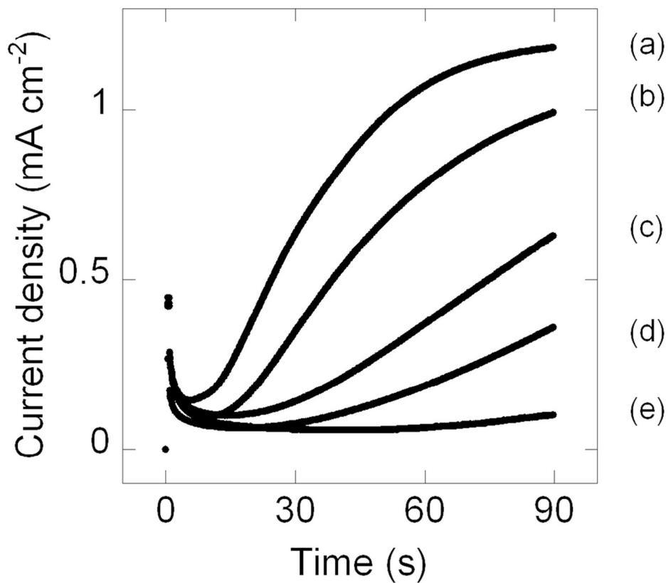
Figure 4. Variations of reduction currents in 0.1 M phosphate buffer containing 5.0 μM Pt complexes and the different concentrations of dsDNA. Concentration of dsDNA: (a) 0, (b) 0.02, (c) 0.2, (d) 2.0 and (e) 20 μg mL<sup>-1</sup>.
