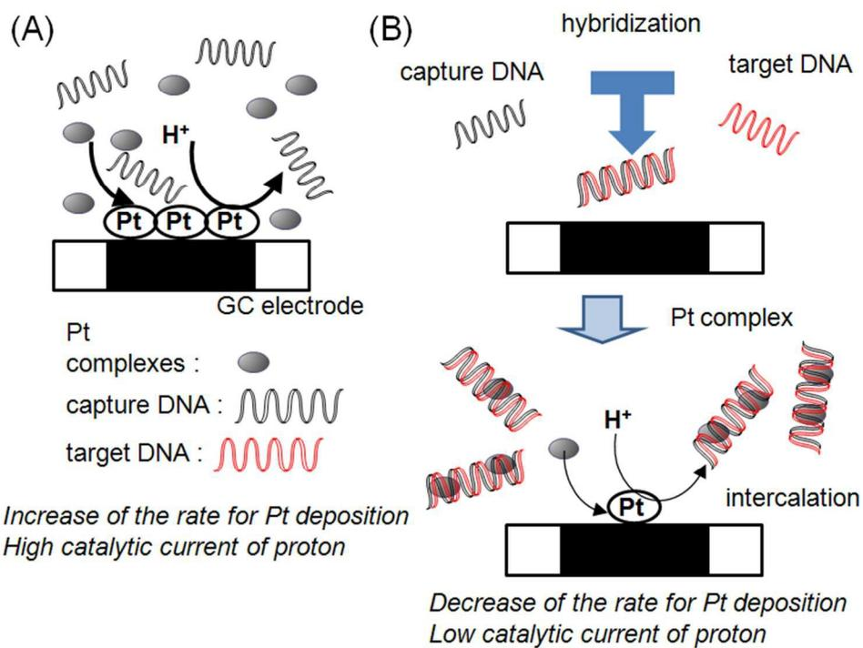
Principle of the electrochemical determination of target DNA with a specific sequence by the intercalation of Pt complexes to the hybridized dsDNA in (A) the absence and (B) the presence of target DNA.
