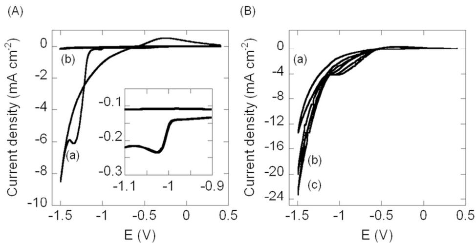
Figure 2. Electrochemical properties for Pt complex on a glassy carbon (GC) electrode by cyclic voltammetry. (A): Cyclic voltammograms of the first cycle on the GC electrode (a) in the presence and (b) in the absence of 0.1 mM Pt complexes. (B): Cyclic voltammograms of (a) second, (b) fourth and (c) sixth scan.
