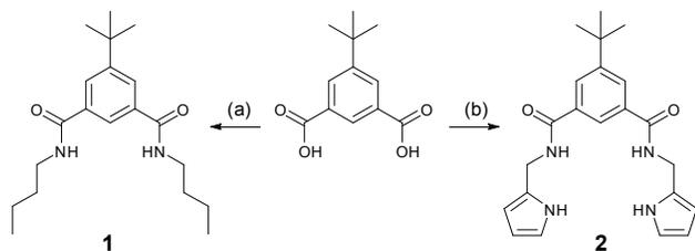
**Scheme 1** Synthesis of receptors **1** and **2**. (a) CDI, *n*-butylamine, DMF, r.t.; (b) i) SOCl<sub>2</sub>; ii) 2-aminomethylpyrrole, Et<sub>3</sub>N, DMF, r.t.
