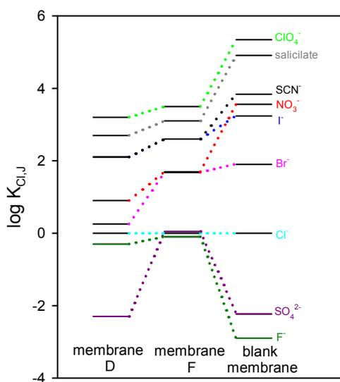
Fig. 5 Pot of the logarithmic selectivity coefficients obtained for membranes containing receptor **1** or receptor **2** (membranes D and F respectively) and for blank membrane (membrane B).
