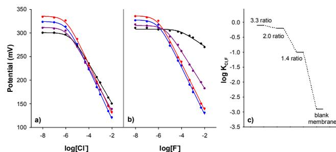
Fig. 4 Calibration graphs for different molar concentrations of (a) chloride and (b) fluoride using membranes with different ionophore-to-ionic ratios. (Membrane B: black; C: purple; D: blue; E: red). (c) Plot of the logarithmic selectivity coefficients for different ionophore-to-ionic additive molar ratio.
