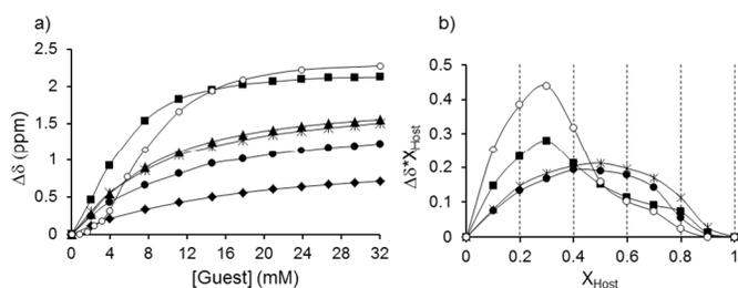
**Fig. 1** a) Titration isotherms and b) Job plots of **1**. ■ F<sup>-</sup>, ◆ Cl<sup>-</sup>, ▲ AcO<sup>-</sup>, \* PhCOO<sup>-</sup>, ● H<sub>2</sub>PO<sub>4</sub><sup>-</sup>, ○ SO<sub>4</sub><sup>2-</sup>, following the NH<sub>amide</sub>-
