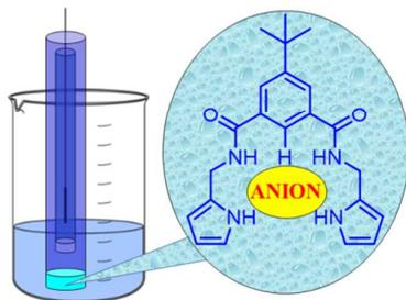
The incorporation of neutral and structurally simple isophthalamide-based receptors into plasticised polymeric membrane anion-selective electrodes has afforded devices with a good sensing ability.
