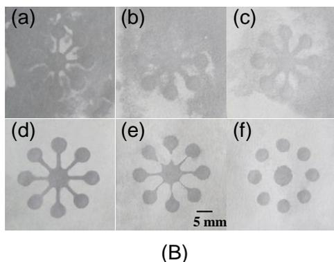
Figure 2(A) Effect of TMOS concentration on the water contact angle on the patterned filter paper. (B) Images obtained by spraying water on the  $\mu$ PAD fabricated with 0.5% (a), 1.0% (b), 1.5% (c), 2.0% (d), 3.0% (e) and 4.0% (f) TMOS-heptane solution. Heating temperature, 100°C; Heating time, 35 min.
