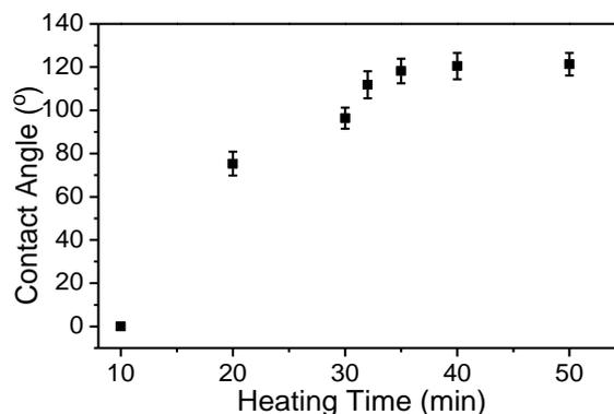
Figure 4 Effect of heating time on the water contact angle on the patterned filter paper. TMOS concentration: 2.0%; Other conditions were the same as Figure 2.
