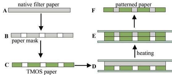
The  $\mu$ PAD was fabricated based on chemical patterning of filter paper by using a paper mask and TMOS solution.
