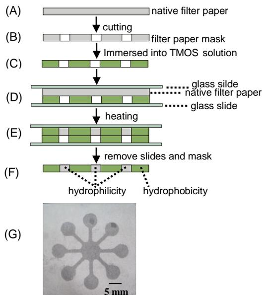
Figure 1 Schematic diagram of fabrication of  $\mu$ PAD. Cross section of (A) the native filter paper, (B) filter paper mask obtained by cutting on the native filter paper, (C) the paper mask penetrated with TMOS solution, (D) the native filter paper sandwiched with two glass slides and a paper mask, (E) the assembly after being heated, and (F) the fabricated  $\mu$ PAD with hydrophilic-hydrophobic contrast. (G) Photograph obtained by spraying water on the fabricated  $\mu$ PAD.
