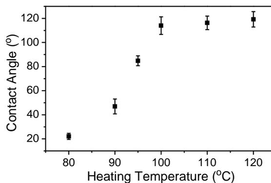
Figure 3 Effect of heating temperature on the water contact angle on the filter paper. TMOS concentration: 2.0%; Other conditions were the same as Figure 2.
