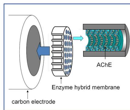
**Figure 3.** Schematic diagram of a working electrode in this study.
