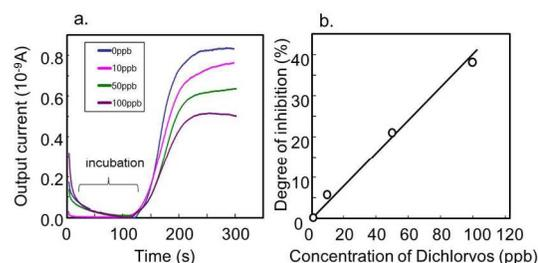
**Figure 10.** a) Current responses of AChE-(F127-MST) in the presence of different concentrations (0, 10, and 100 ppb) of inhibitor, i.e., dichlorvos, and b) degree of inhibition against concentration of dichlorvos. Measurements were done in phosphate buffer (pH 7.4) by injecting acetylthiocholine solutions.
