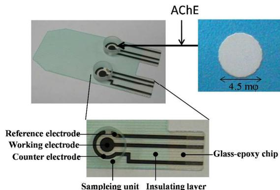
**Figure 7.** The manufactured screen-printed carbon electrode containing TCNQ on a glass-epoxy substrate.
