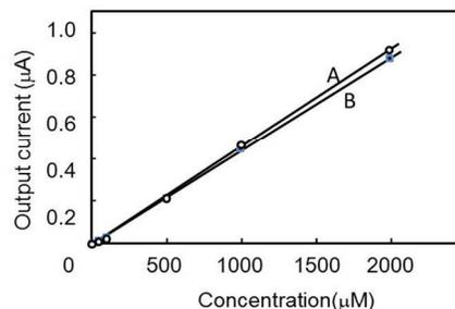
**Figure 9.** Output current against the different concentration of acetylthiocholine at each right (A)-and-left (B) electrodes.
