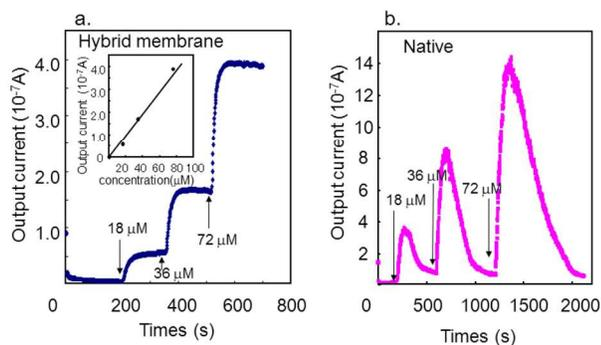
**Figure 4.** Typical responses of (a) AChE-(F127-MST) (0.014 mg/ 1.8 mg) and (b) the native AChE (0.015 mg) to the injections of acetylthiocholine solutions (18, 36 and 72  $\mu$ M) at a constant potential of  $E_{app} = 0.2$  V. The electrolytes comprise 0.5 mM TCNQ in 90  $\mu$ l of a phosphate buffer (pH 7.4).
