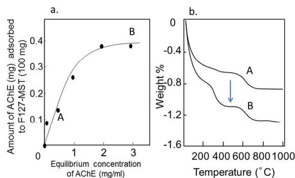
**Figure 2.** a) Spectrophotometrically measured adsorption of AChE onto F127-MST with respect to the equilibrium concentrations of AChE. b) TG-DTA curves for AChE-(F127-MST), where the amounts of AChE adsorbed to F127-MST (100 mg) for A and B are 0.14 and 0.38 mg, respectively.
