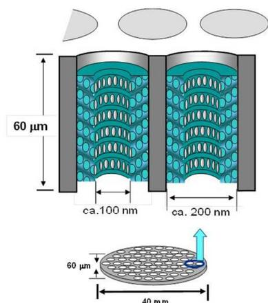
**Figure 1.** Schematic illustrations of the anodic alumina membrane and the assembly of silica-surfactant nanochannels (channel diameter = 13 nm) formed inside the columnar alumina pore (pore diameter = 200 nm).
