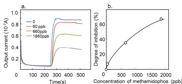
**Figure 6.** Current responses of AChE-(F127-MST) in the presence of different concentrations (0, 60, 660, and 1860 ppb) of inhibitor, methamidophos. and b) degree of inhibition against concentration of methamidophos. Measurements were done in 0.5 mM TCNQ / phosphate buffer (pH 7.4) by injecting acetylthiocholine solutions (36  $\mu$ M).
