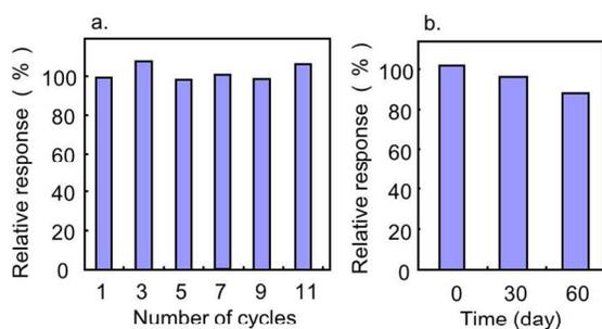
**Figure 5.** a) Relative current response of AChE-(F127-MST) (0.014 mg/1.8 mg) under the repeated use, and b) under the long-term storage stability (30 and 60 days). The current responses were measured by injections of a acetylthiocholine solutions (36  $\mu$ M) at a constant potential of  $E_{app} = 0.2$  V. The electrolytes comprise 0.5 mM TCNQ in 90  $\mu$ l of a phosphate buffer (pH 7.4).
