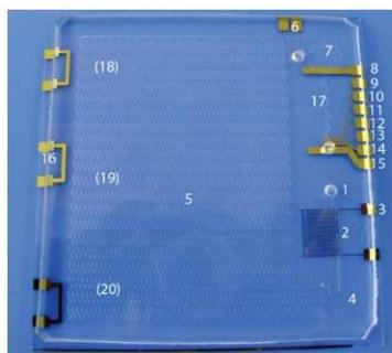
**Figure 10.** The PCR microdevice showing glass substrate, ITO microheaters, PDMS mold containing microchannels, gold microelectrodes for cell lysis, PCR amplification and CE-AD operation [100].
