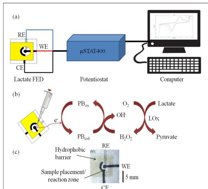
Fig.2 Overview of FED technology. (a) The instrumental setup for lactate determination. (b) The reaction that occurs at the C-PB/LOx electrodes of the FED. (c) Picture of the fabricated FED (15 x 15 mm). RE, reference electrode; WE, working electrode; CE, counter electrode.
