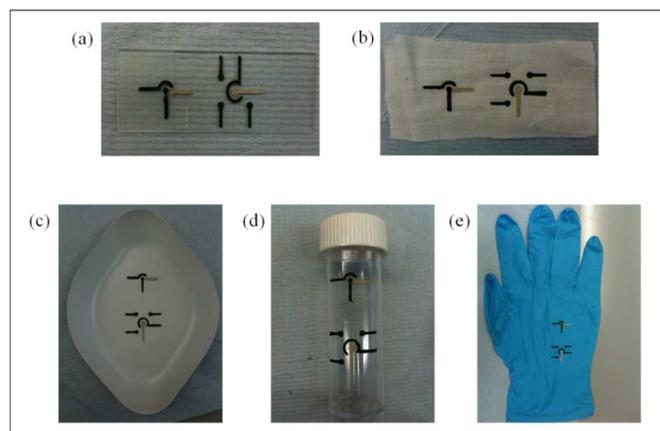
Fig.3 Electrodes patterned on: (a) Glass microscope slide. (b) Cotton fabric. (c) Plastic weighing boat. (d) On the outer surface of a polypropylene centrifuge tube. (e) Nitrile glove.
