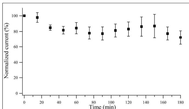
Fig.6 Stability of the lactate FED to 0.5 mM lactate over a 3 h operation with repetitive measurement carried out at 15 min intervals. The initial current at t=0 min is normalised to 100%. Error bars =  $\pm$  SEM (n = 3).
