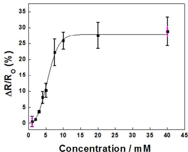
Fig. 6. Response of the PABA coated SWNT sensors towards D-glucose at pH of 7.4 with the corresponding sigmoidal fit.
