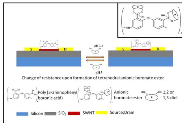
Fig. 1. Schematics of the chemiresistive PABA coated SWNT sensor. Structure of the anionic boronate ester (inset).
