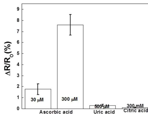
Fig. 8. Response of PABA coated SWNT sensors towards 30  $\mu$ M ascorbic acid, 300  $\mu$ M ascorbic acid, 500  $\mu$ M uric acid and 300 mM citric acid.
