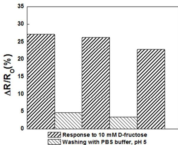
Fig. 7. Response of the PABA coated SWNT sensors towards 10 mM D-fructose and subsequent regeneration by washing with buffer at pH of 5.
