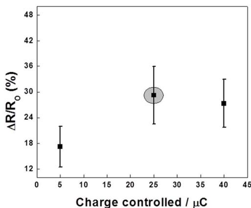
Fig. 4. Response of PABA coated SWNT sensors electropolymerized at 5, 25 and 40  $\mu\text{C}$  charge towards 10 mM D-fructose.
