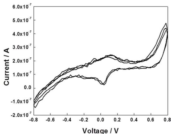
Fig. 3. CV of PABA coated SWNT device in 10X PBS plus 300 mM NaF; pH 5.0. Scan rate: 100 mV s<sup>-1</sup>
