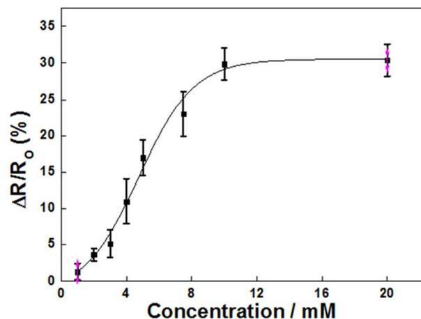
Fig. 5. Response of the PABA coated SWNT sensors towards D-fructose at pH of 7.4 with the corresponding sigmoidal fit.
