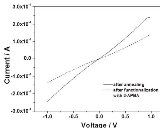
Fig. 2.  $I_{\text{DS}}$  vs.  $V_{\text{DS}}$  of AC dielectrophoretically aligned SWNTs network before and after electropolymerization of 3-APBA.
