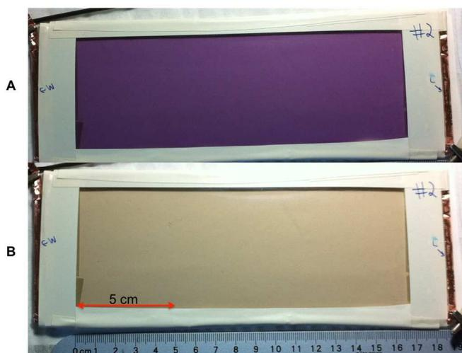
Fig. 1 (A) Colored state and (B) Bleached state for an electrochromic window of 105cm<sup>2</sup> active area using the *in situ* procedure with 2.5 wt% ProDOT-Me<sub>2</sub> in the electrolyte gel.
