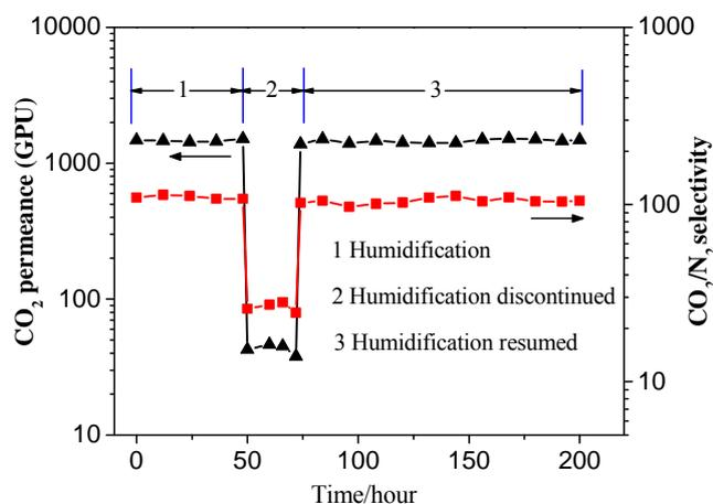
**Figure 4.** Separation performance stability of PEIE-HT membrane. Wet coating thickness: 50 $\mu$ m; Feed gas: 15vol% CO<sub>2</sub> and 85vol% N<sub>2</sub>, 0.2MPa, 298.15K.
