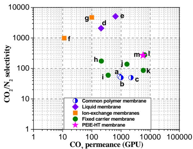
**Figure 3.** Performance comparison of various membranes. Detailed data list in Supplementary Table S2.
