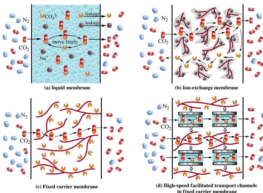
**Scheme 1.** Schematic of  $\text{CO}_2$  transport mechanisms in different membrane (a)  $\text{Na}_2\text{CO}_3$  liquid membrane; (b) Ion-exchange membrane; (c) fixed carrier membrane; (d) high-speed facilitated transport channels grafted in fixed carrier membrane.
