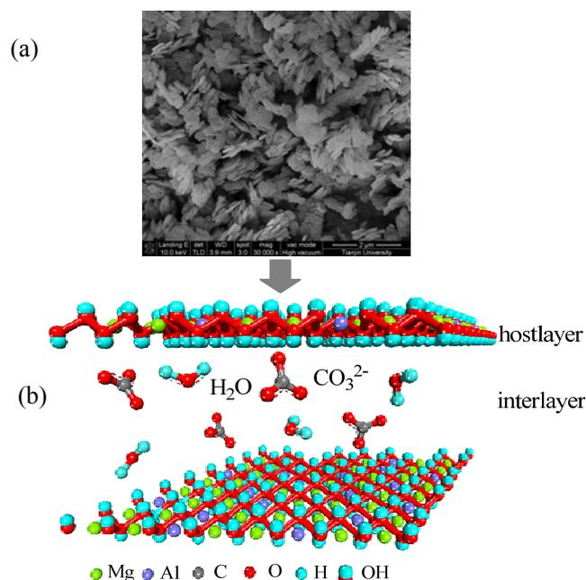
**Scheme 2.** Structure of HT (a) SEM image of HT synthesized in this paper, size: about 110nm; (b) Schematic drawing of HT.
