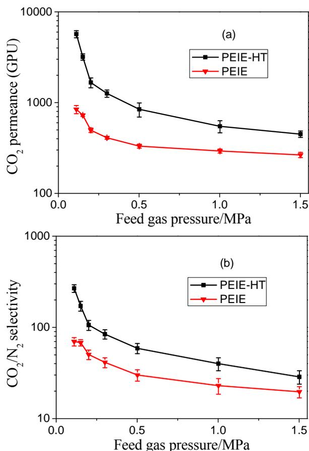
**Figure 2.** The CO<sub>2</sub>/N<sub>2</sub> separation performance of PEIE-HT membrane and PEIE membrane (a) CO<sub>2</sub> permeance; (b) CO<sub>2</sub>/N<sub>2</sub> selectivity. Wet coating thickness: 50 μm; Feed gas: 15 vol% CO<sub>2</sub> and 85 vol% N<sub>2</sub>. 298.15K.
