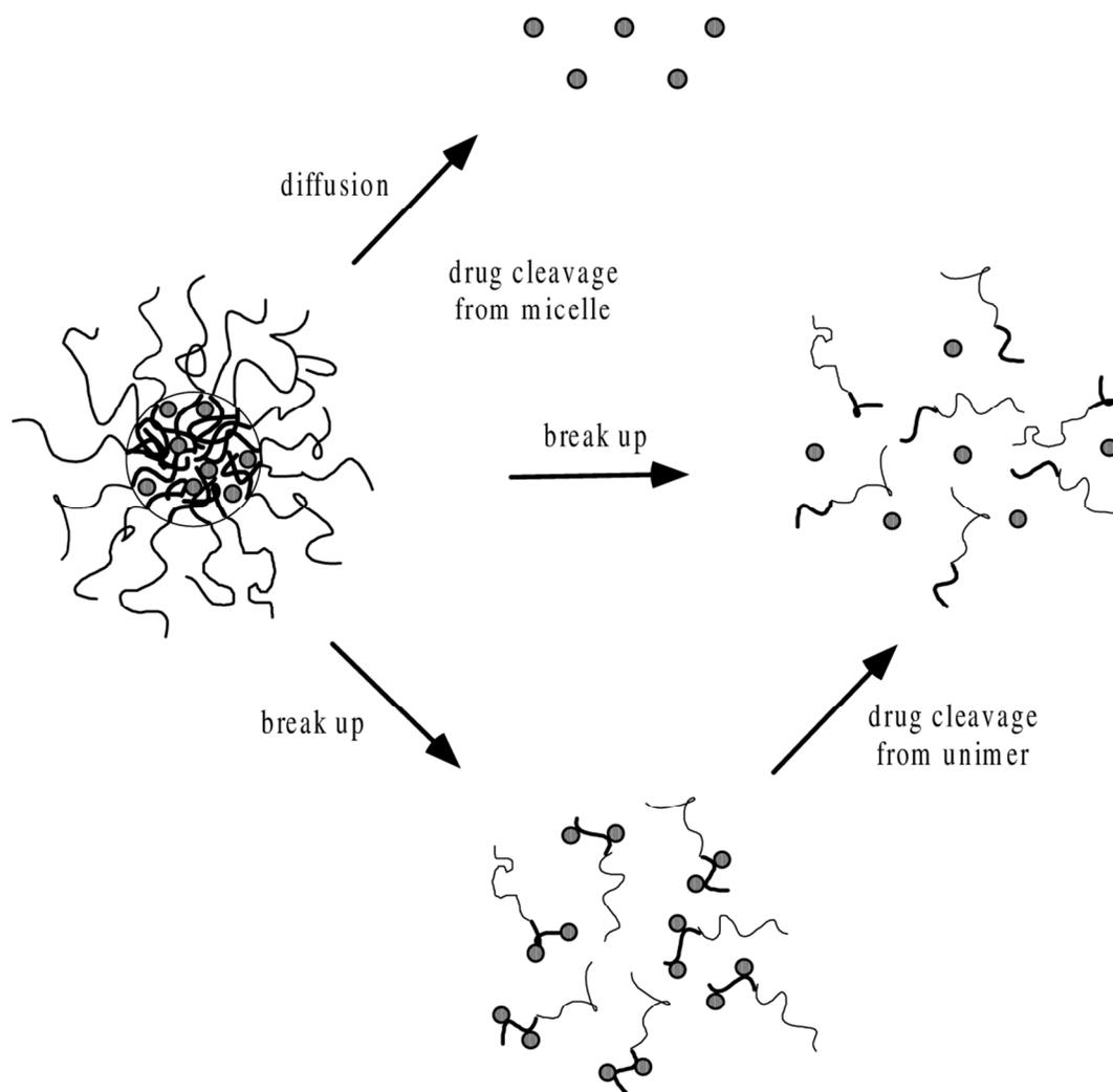
**Fig.4.** Mechanisms of drug release from polymeric micelles [8,88].
