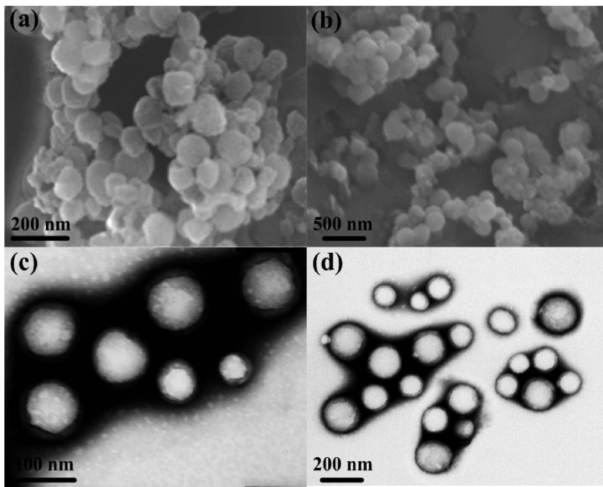
**Fig. 1.** SEM and TEM images of blank (a, c) and IBU-loaded (b,d) P(MMA3k-co-MAA4.5k)-b-PPEGMA5k assembled micelles [26].
