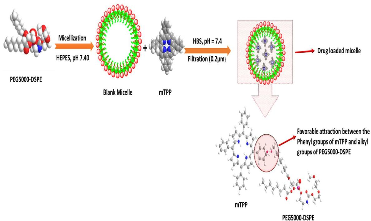
**Fig.2.** Schematic of the decrease in micellar size after drug incorporation. PEG5000-DSPE represents poly ethylene glycol-distearoyl phosphatidyl ethanolamine, HEPES (4-(2-hydroxyethyl)-1-piperazine ethane sulfonic acid), mTPP (meso-tetraphenyl porphine) and HBS (HEPES Buffered Saline).
