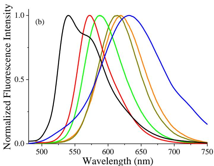
**Figure 5.** Normalized absorption (a) and emission (b) spectra of curcumin-BF<sub>2</sub> **1k** in six different solvents at room temperature. Cyclohexane (black), toluene (red), tetrahydrofuran (green), methanol (blue), acetonitrile (orange) and dichloromethane (dark yellow).
