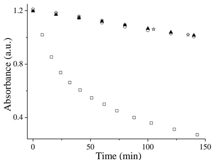
**Figure 6.** Comparison of the photostability of curcumin-BF<sub>2</sub> complexes ( $2 \times 10^{-5}$  M) **1d** (☆), **1k** (○), **1e** (△) and Rose Bengal ( $4 \times 10^{-5}$  M, □) in toluene (1% DMF) under continuous irradiation with a 500 W Xe lamp.
