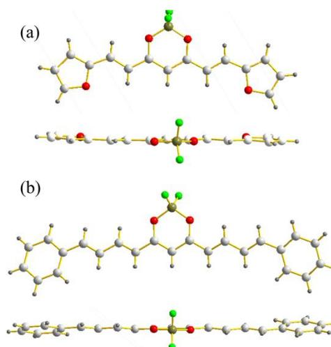
**Figure 2.** Top view (top) and side view (bottom) of X-ray structures of curcumin BF<sub>2</sub> complexes **1i** (a) and **1j** (b). C, light gray; H, gray; O, red; B, dark yellow; F, light green.
