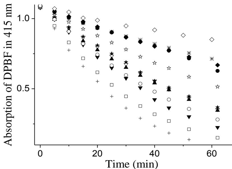
**Figure 8.** Comparative DPBF (initial concentration at  $5 \times 10^{-5}$  M) degradation profiles in toluene (1% DMF) by curcumin- $\text{BF}_2$  complexes ( $1 \times 10^{-6}$  M): **1b** (●), **1c** (☆), **1d** (+), **1e** (▼), **1f** (○), **1g** (◆), **1h** (▽), **1i** (▲), **1j** (★), **1k** (□), **3b** (\*), and **3c** (◇). Filtered light  $> 455$  nm used.
