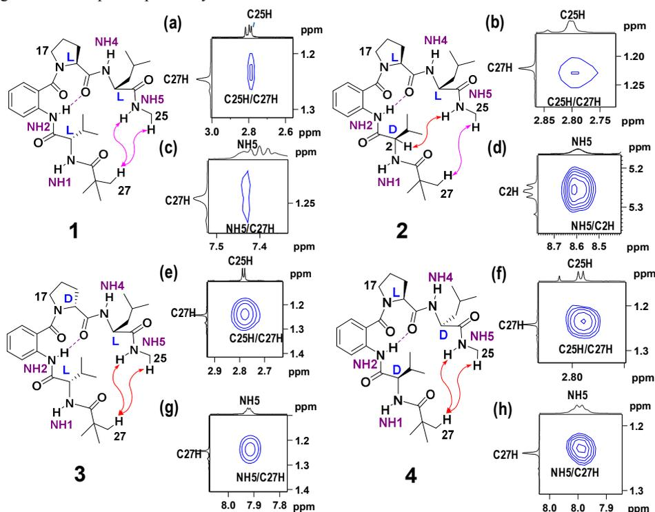
**Figure 4.** Selected nOe extracts from the 2D NOESY data of **1-4** (CDCl<sub>3</sub>, 400/500 MHz, 298 K): (a), (b), (e) & (f) Piv vs methylamide -CH<sub>3</sub>; (c), (g) & (h) Piv vs NH<sub>5</sub>; (d) NH<sub>5</sub> vs Val $\alpha$ H.
