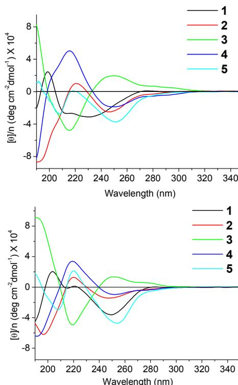
50 **Figure 6.** Comparison of CD spectra of tetramer analogues **1-5** in TFE (top) and **1-5** in acetonitrile (bottom), respectively (0.1 mM).
