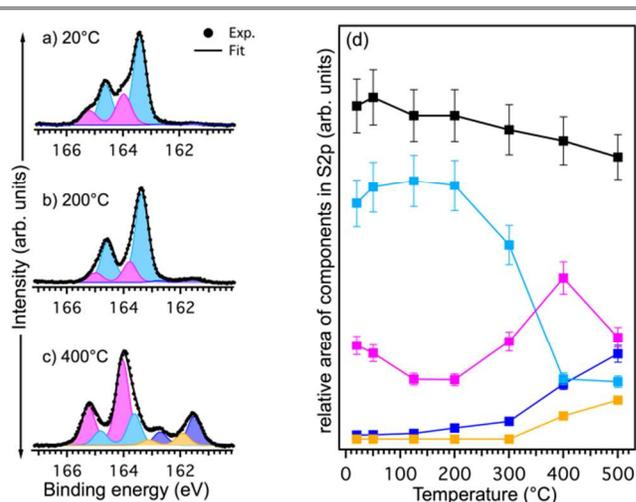
**Figure 7.** S 2p core level for Ag(111). (a) Sample after deposition of TBTTA without annealing. (b) After annealing to 300 °C and (c) after annealing to 400 °C. (d) Area of the different contributions after deconvolution for all annealing temperatures.
