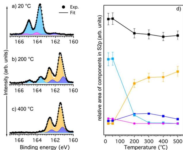
**Figure 4.** S 2p core level spectra for TBTTA on Cu(111). (a) After deposition of TBTTA without annealing. (b) After annealing to 200 °C, and (c) after annealing to 400 °C for 10 minutes. (d) Areas of the different contributions after deconvolution for all annealing temperatures.
