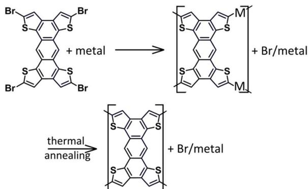
**Scheme 1.** TBTTA in the surface-confined Ullmann reaction from precursor molecule to organometallic intermediate, and to  $\pi$ -conjugated covalent polymer.
