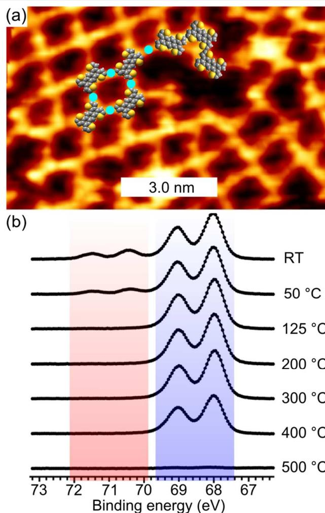
**Figure 5.** (a) STM image of the 2D network on Ag(111) ( $U_{\text{bias}} = -758$  mV,  $I_{\text{tunnel}} = 0.877$  nA). (b) Core-level spectra of the Br 3d level on Ag(111) at room temperature and various annealing temperatures up to 500 °C.
