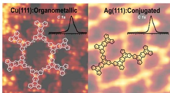
We present an STM and XPS study on the synthesis of organometallic and covalent polymeric molecular networks and elucidate the role of the supporting substrate on their thermal stability.
