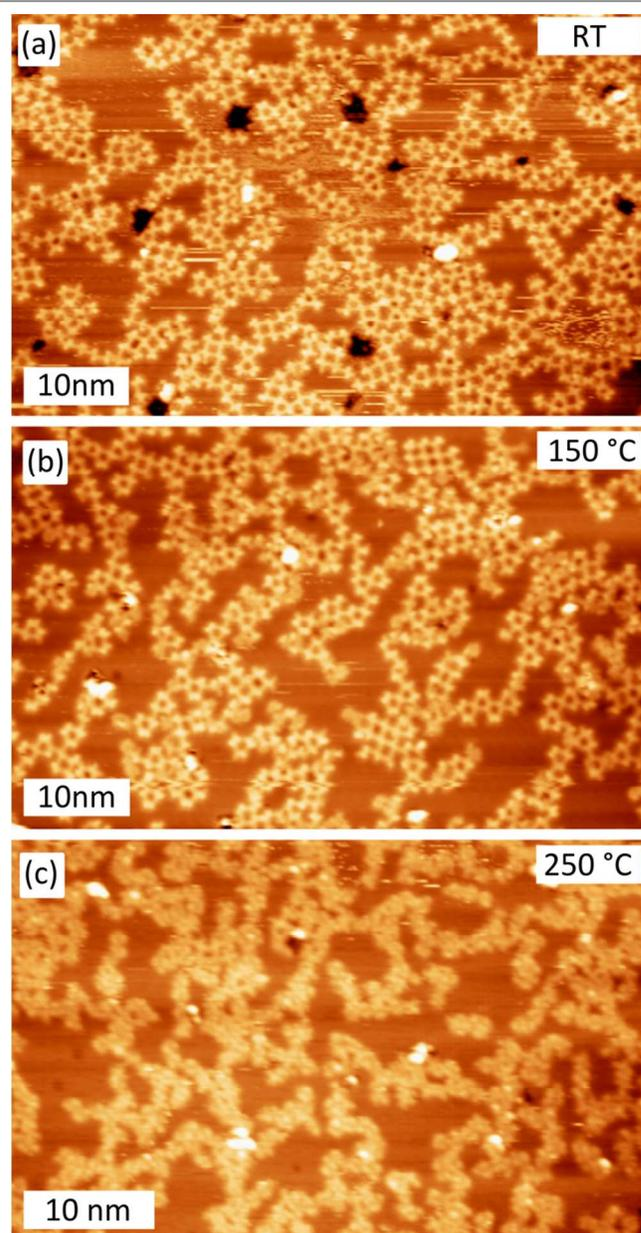
**Figure 1.** Overview images of TBTTA on Cu(111) as deposited at (a) room temperature ( $U_{\text{bias}} = -2000$  mV,  $I_{\text{tunnel}} = 0.590$  nA), (b) after annealing to 150 °C ( $U_{\text{bias}} = -1600$  mV,  $I_{\text{tunnel}} = 0.430$  nA), and (c) after annealing to 250 °C ( $U_{\text{bias}} = -1900$  mV,  $I_{\text{tunnel}} = 0.370$  nA) for 10 minutes.
