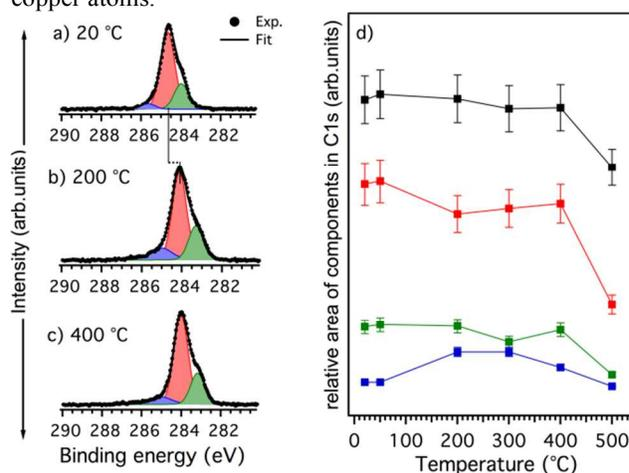
**Figure 3.** C 1s core level on Cu(111) for (a) room temperature as deposited, (b) after annealing to 200 °C and (c) after annealing to 400 °C for 10 minutes. The evolution of each contribution with annealing temperature is plotted in (d). (total signal: black curve, Voigt fits in blue, red, and green).
