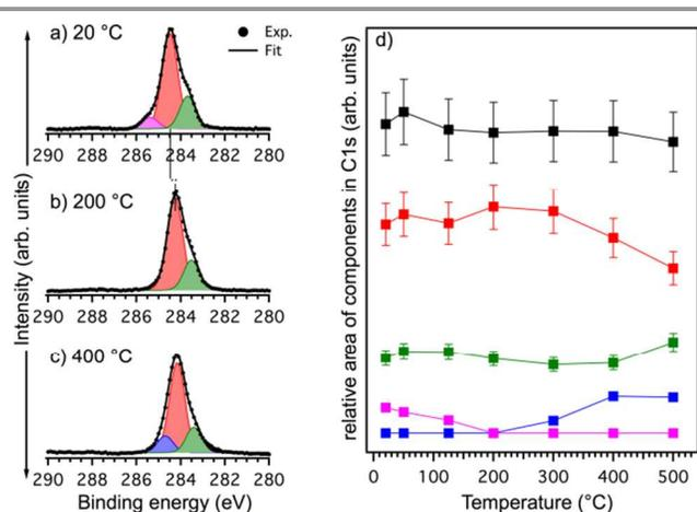
**Figure 6.** C 1s core level on Ag (111) at (a) room temperature and after annealing to (b) 200 °C and (c) 400 °C. (d) Peak-area evolution as a function of annealing temperature.
