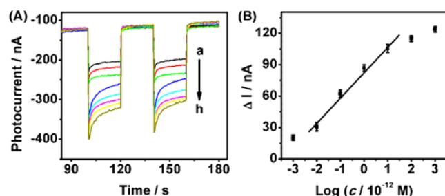
Fig. 7 (A) Photocurrent responses of the biosensor at different concentrations of target DNA. (B) The corresponding calibration curve ( $\Delta I = I - I_0$ ,  $I_0$  and  $I$  are the photocurrents of capture DNA/CdTe/ZnO/ITO without and with target DNA, respectively).
