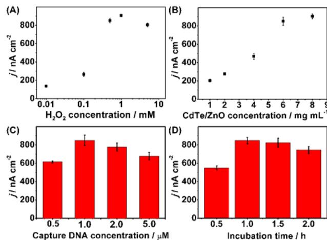
**Fig. 6** Effects of (A) H<sub>2</sub>O<sub>2</sub> concentration, (B) CdTe/ZnO concentration, (C) capture DNA concentration and (D) incubation time on photocurrent responses of the biosensor (error bar results from three independent electrodes).
