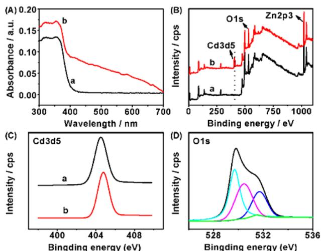
**Fig. 3** (A) UV-Vis, (B) survey and (C) Cd3d<sub>5</sub> XPS spectra of porous ZnO nanosheets (a) and CdTe/ZnO nanohybrids (b). (D) is O1s XPS spectra of CdTe/ZnO nanohybrids.
