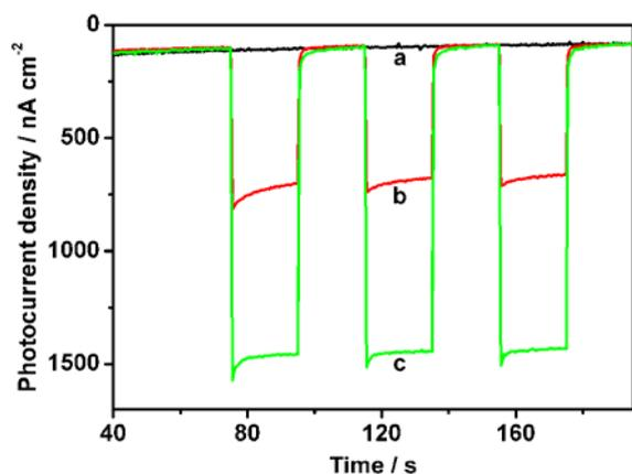
**Fig. 5** Photocurrent responses of (a) ZnO, (b) CdTe, and (c) CdTe/ZnO modified ITO electrodes in 0.1 M Tris-HCl (pH=7.4) containing 0.5 mM H<sub>2</sub>O<sub>2</sub>. Light excitation of 505 nm is switched every 20 s and the applied potential is -0.20 V.
