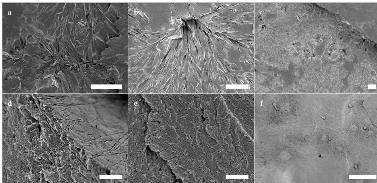
**Figure 2** SEM images showing the different pore morphologies resulting from the imprinting of different concentrations of gelator: a) 1 % w/v **1** [5  $\mu\text{m}$ ] b) 5 % w/v **1** [5  $\mu\text{m}$ ] c) 10 % w/v **1** [10  $\mu\text{m}$ ], d) 5 % w/v **2** [500 nm] e) 5 % w/v **2** [500 nm] f) 10 % w/v **2** [20  $\mu\text{m}$ ] with distance denoted by white scale bar given in square brackets
