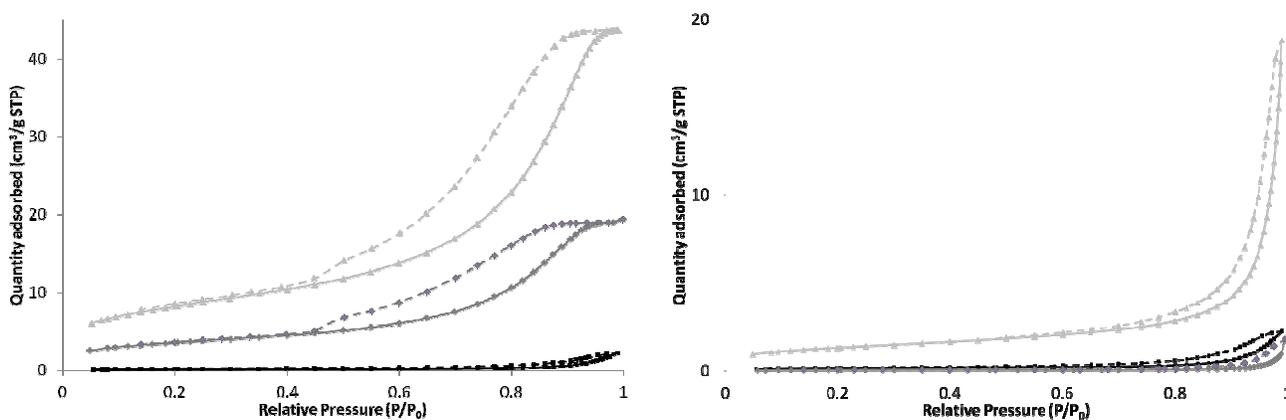
**Figure 3** BET isotherm showing adsorption (solid) and desorption (dashed) isotherms for washed polymer samples formed by 1 % w/v (black), 5 % w/v (grey), 10 % w/v (light grey) of gelators **1** (a) and **2** (b)
