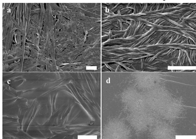
**Figure 1** SEM images showing a) 5 % w/v xerogel of **1** [1  $\mu$ m] b) 2 % w/v xerogel of **2** [500 nm] c) unwashed composite of 10 % w/v **1** in 1:1 MMA:EGDMA [5  $\mu$ m] d) unwashed composite of 5 % w/v **2** in 1:1 MMA:EGDMA [5  $\mu$ m] with distance denoted by white scale bar given in square brackets
