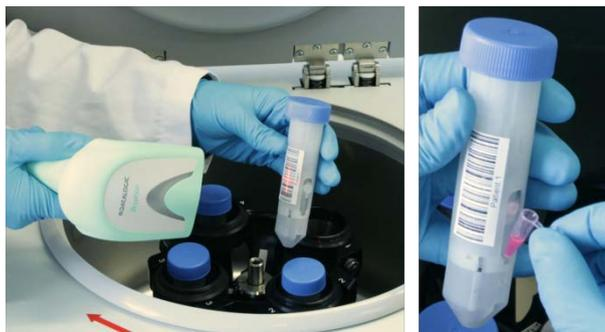
**Figure 1.** LabTube workflow. LabTube cartridge and centrifuge with swing-bucket rotor. If desired, a barcode scanner can be used for transfer of the assay specific centrifugation-time-protocol. After protocol completion, the eluate (colored in pink) is obtained in a detachable collection tube.
