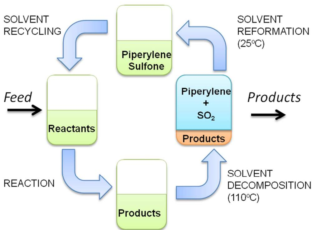
**Figure 34.** Recycling and reformation process of piperylene sulfone.
