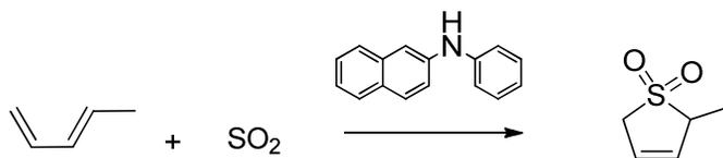
**Figure 31.** Synthesis of piperylene sulfone.
