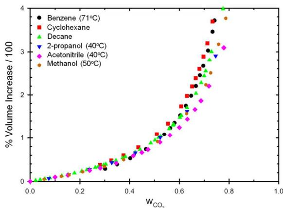
**Figure 14.** Volume expansion with  $\text{CO}_2$  for benzene, cyclohexane, decane, 2-propanol, acetonitrile and methanol.
