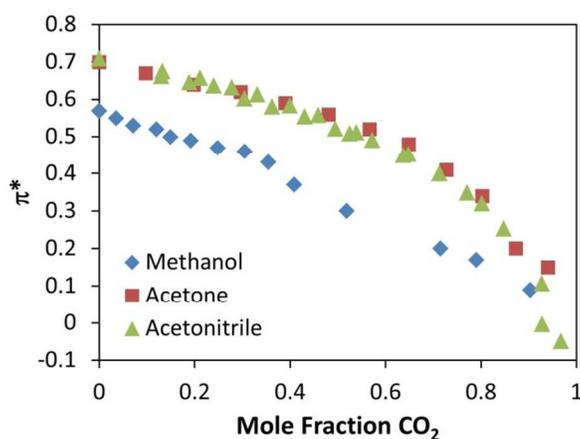
**Figure 15.** Experimental  $\pi^*$  values for gas-expanded methanol (using 4-nitroanisole),<sup>65</sup> acetone (N,N-dimethyl-4-nitroaniline)<sup>65</sup> and acetonitrile (using 4-nitro-anisole)<sup>63,64,66</sup> as a function of  $\text{CO}_2$  mol fraction at 40 °C.
