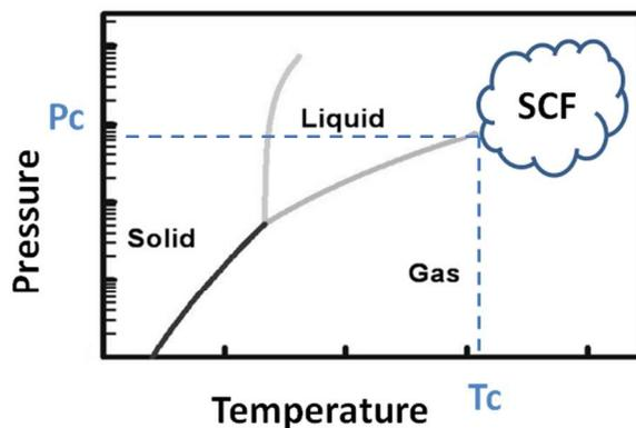
**Figure 2.** General phase diagram for supercritical fluids.
