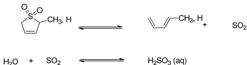
**Figure 37.** Formation of sulfurous acid through equilibrium reaction between SO<sub>2</sub> and water for butadiene sulfone (H) or piperylene sulfone (CH<sub>3</sub>).
