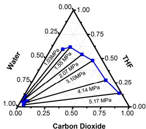
**Figure 22.** Ternary diagram of the system THF/Water/CO<sub>2</sub> at 25 °C, showing the liquid-liquid equilibrium at various CO<sub>2</sub> pressures.
