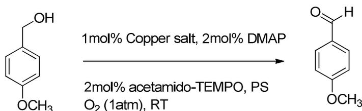
**Figure 35.** Oxidation of 4-methoxybenzyl alcohol in piperylene sulfone.
