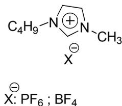
**Figure 39.** Structure of BMIM-PF<sub>6</sub> & BMIM-BF<sub>4</sub>
