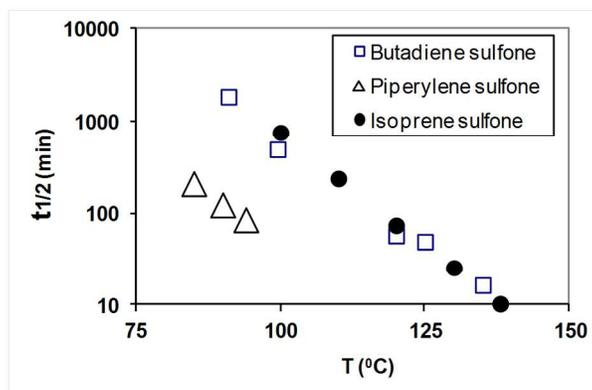
**Figure 33.** Decomposition half-life of ■ = butadiene sulfone, ● = isoprene sulfone, and Δ = piperylene sulfone.<sup>145</sup>
