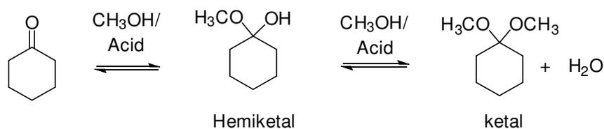
**Figure 18.** Ketal formation in gas-expanded alcohol.
