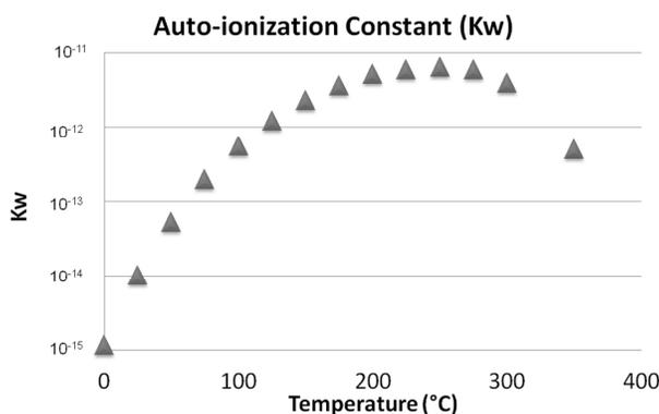
**Figure 29.** Dissociation constant of water as a function of temperature from 0-350°C.
