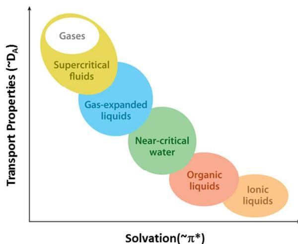
**Figure 1.** Compromise of transport ability and solvent power for various types of solvents.
