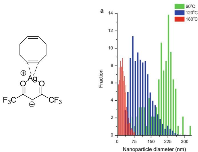
**Figure 13.** Structure of the precursor 1,1,1,5,5,5-hexafluoroacetylacetonate cyclooctadiene  $\text{Ag}(\text{hfac})(\text{COD})$  and particle size distribution of silver nanoparticles deposited from  $\text{scCO}_2$  onto a HCl treated silicon surface. Reprinted with kind permission from Springer Science and Business Media (M. Casciato, G. Levitin, D. Hess and M. Grover, *J. Nanopart. Res.*, 2012, 14, 1-15).<sup>17</sup>
