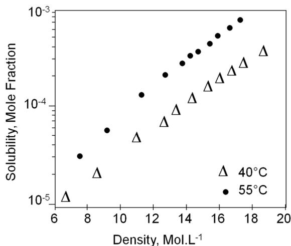
**Figure 4.** Solubility of salicylic acid (2-hydroxybenzoic acid) in scCO<sub>2</sub>.
