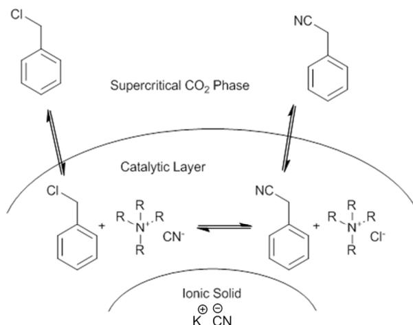
**Figure 7.** Mechanism of PTC reaction in scCO<sub>2</sub>.<sup>18</sup>
