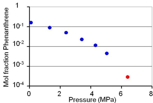
**Figure 16.** Solubility of phenanthrene in gas expanded acetone as a function of CO<sub>2</sub> pressure.
