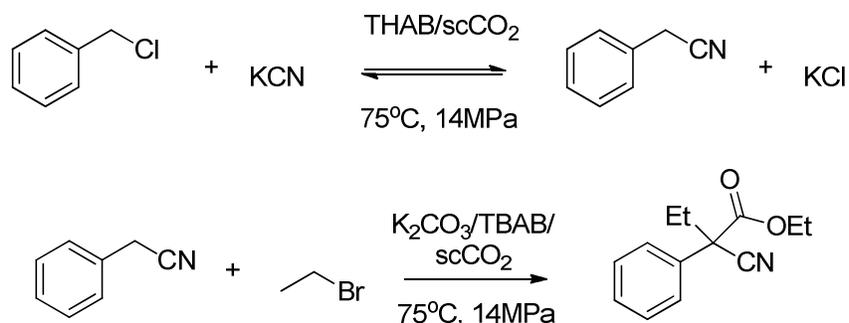
**Figure 6.** Example reactions in supercritical fluids: substitution of benzyl chloride with potassium cyanide to form phenylacetonitrile in scCO<sub>2</sub> (top), formation of α-phenyl-α-ethylcyanoacetate during the alkylation of phenylacetonitrile with scCO<sub>2</sub> (bottom).
