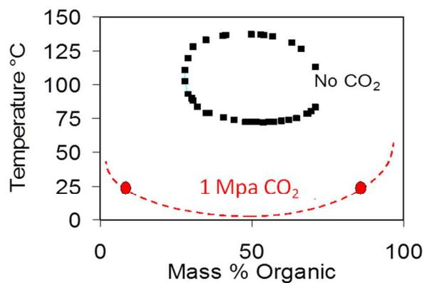
**Figure 21.** Liquid-liquid phase boundaries for THF/Water with and without CO<sub>2</sub>.
