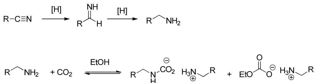
**Figure 20.** Hydrogenation of nitriles to form primary amines and the *in situ* protection of the synthesized amine with CO<sub>2</sub>.
