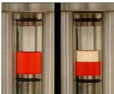
**Figure 23.** Water-THF-CO<sub>2</sub> Equilibria. Left: No CO<sub>2</sub>, a single phase. Right: 2 MPa of CO<sub>2</sub>, two liquid phases with dye partitioning >10<sup>6</sup>.
