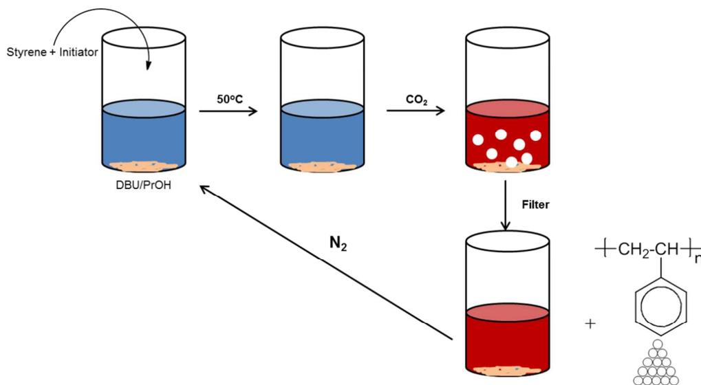
**Figure 41.** Polymerization of styrene in DBU/Propanol RevIL. Blue indicates molecular liquid and red indicates ionic liquid.
