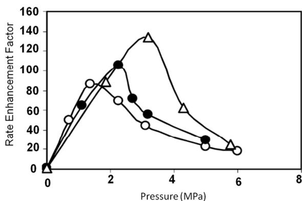
**Figure 19.** Enhancement of rate constant for cyclohexanone ketal formation in gas expanded methanol. Symbols key: (○) 25 °C, (●) 40 °C and (△) 50 °C. Reprinted with permission from (X. Xie, C. L. Liotta and C. A. Eckert, *Ind. Eng. Chem. Res.*, 2004, 43, 2605-2609). Copyright (2004) American Chemical Society.<sup>77</sup>
