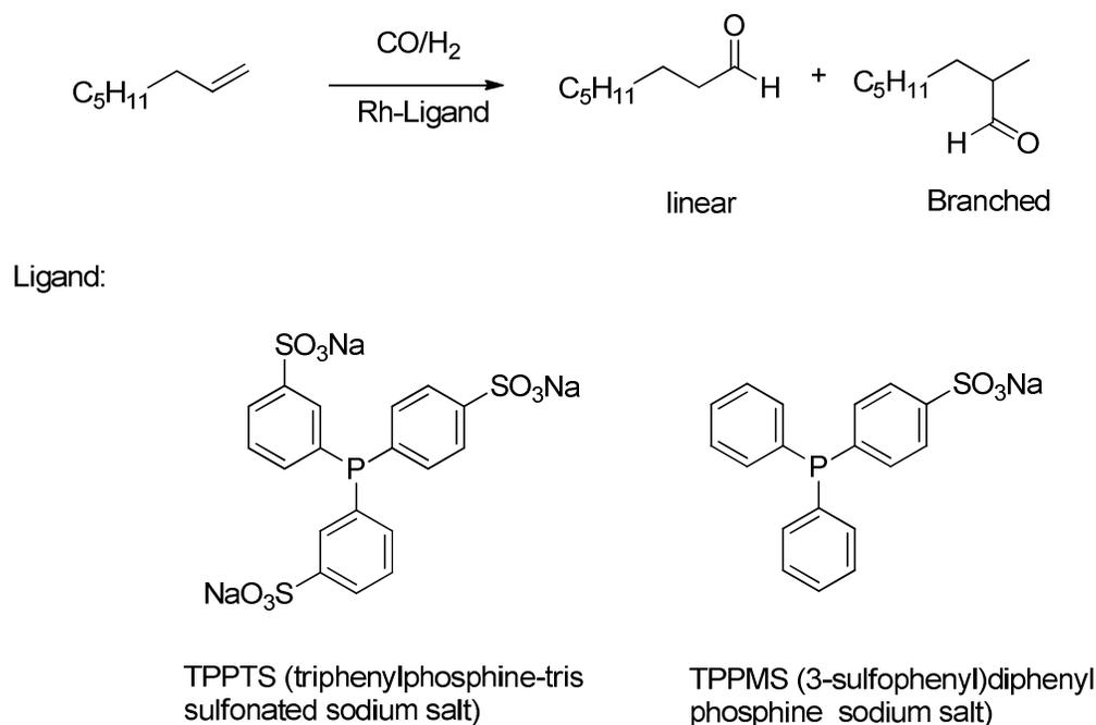
**Figure 25.** Hydroformylation of 1-octene to form 1-nonanal (linear product) and 2-methyloctanal (branched product).
