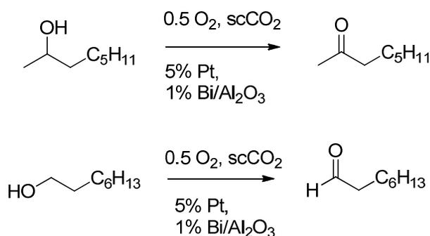
**Figure 12.** Oxidation of 2-octanol and 1-octanol in scCO<sub>2</sub>.<sup>19</sup>
