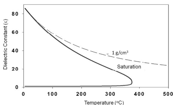
**Figure 28.** Dielectric constant of water as a function of temperature from 0-500°C. Correlation from Uematsu and Franck<sup>101</sup>.
