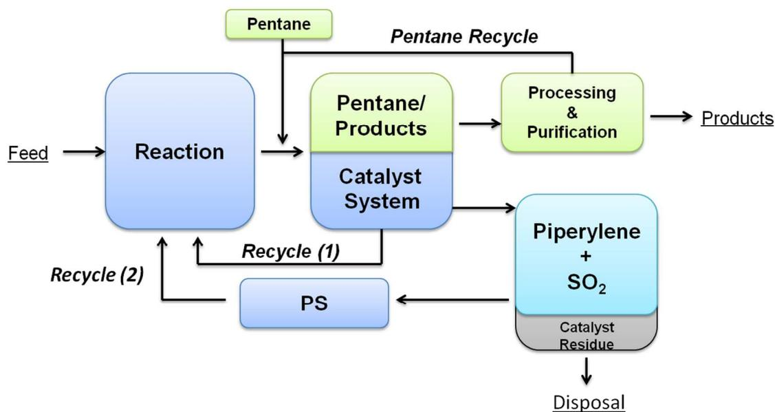
**Figure 36.** Process schematic for the PS-mediated oxidations of alcohols.
