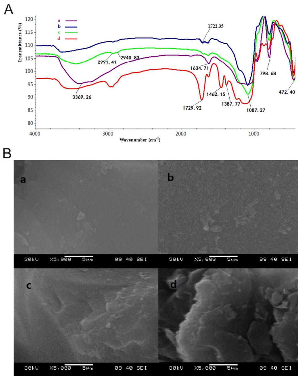
Fig. 1. FT-IR spectra (A) of activated silica-gel (a), CDS (b), DCDS (c) and MIP-2 (d). SEM images (B) of activated silica gel (a), DCDS (b), NIP-2 (c) and MIP-2 (d).
