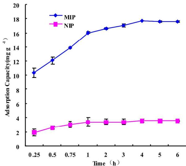
Fig. 3. Adsorption kinetic curves of MIP-2 and NIP-2. Experimental conditions: 0.12 mmol L<sup>-1</sup> Dufulin in binding medium of 5 mL methanol/water (30/70, v/v) with 10.0 mg MIP-2 or NIP-2 for certain hours, respectively. The measurements were repeated three times.
