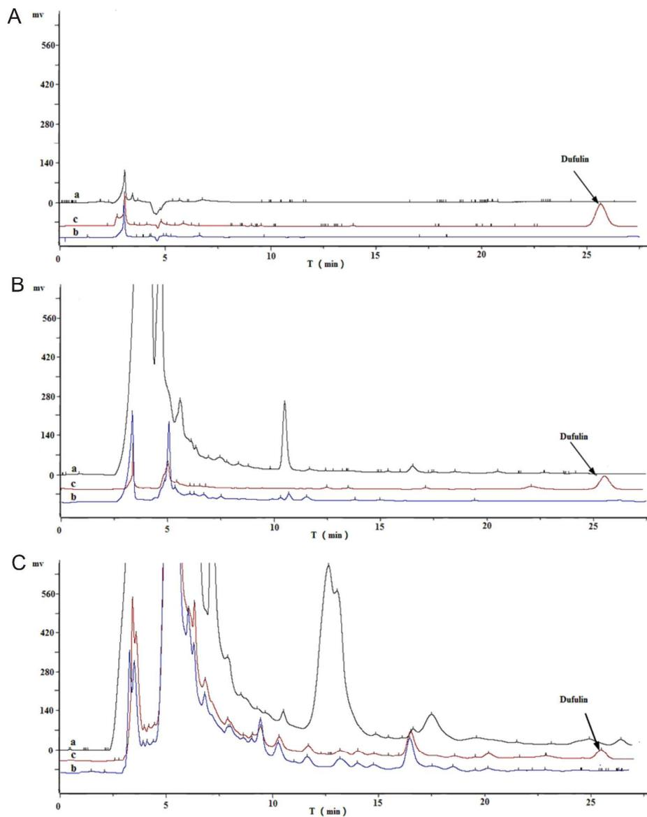
Fig. 5. Chromatograms of spiked Dufulin ( $0.5 \text{ mg L}^{-1}$ ) in water (A), soil (B) and wheat (C) samples: blank sample by direct injection (a); blank sample with MIP-SPE (b); spiked sample with MIP-SPE (c).
