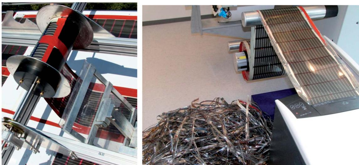
Fig. 2 Left. The start of the de-installation of a 100 m stretch of a flexible organic solar cell at  $200 \text{ m min}^{-1}$ . Right. Roll-to-shredding with continuous cutting of a roll of used OPV. The pile of shreds ready for silver recovery represents 10 m solar foil (width of 0.305 m).
