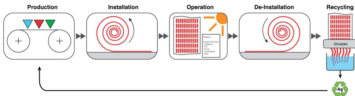
Fig. 1 Complete life cycle of OPV from manufacture of solar cell modules through their deployment in a solar park, operation until they have produced the same energy that was invested in their fabrication to the de-installation, reclaim and decommissioning once they have paid this energy back to finally the recycling of silver.
