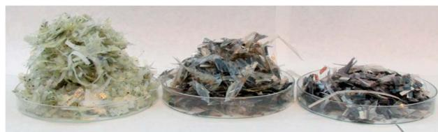
Fig. 3 Photograph of the remaining shredded pieces after the  $\text{HNO}_3$  treatment from the ‘non-delaminated’ experiment (from left to right: 14.2 M, 4.74 M and 1.42 M). Besides the apparent difference in color there is a distinct difference in the subsequent volumes of the piles after the acid treatment. The volume differences are the result of different extents of delamination caused by the acid.
