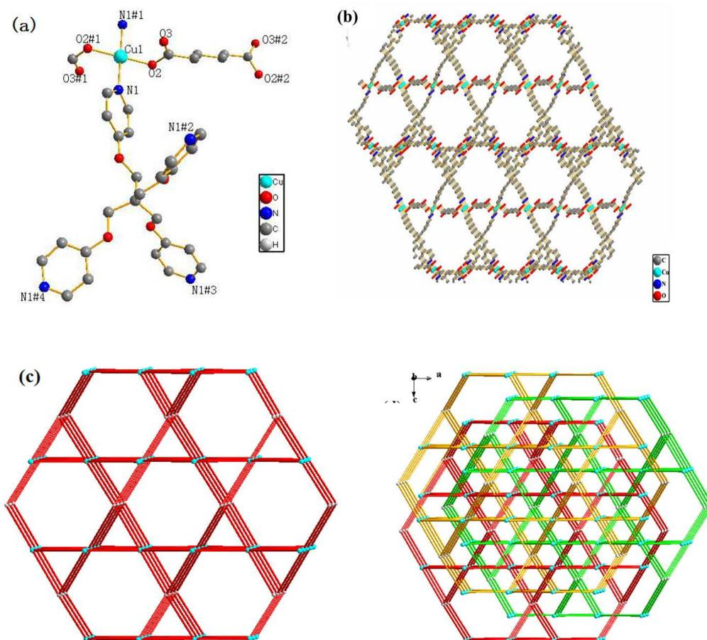
**Figure 1.** (a) Coordination environment of compound **1**. The hydrogen atoms are omitted for clarity (50% ellipsoid probability). Symmetry codes: #1 =  $1 - x, 1 - y, -z$ ; #2 =  $1.5 - x, 0.5 - y, z$ ; #3 =  $1.5 - x, 1.5 - y, z$ ; #4 =  $1.5 - y, x, 1.5 - z$ ; #5 =  $y, 1.5 - x, 1.5 - z$ . (b) Views of the 3D network along the b axis. (c) Schematic view of topology (left) and 3-fold interpenetrating structure (right).
