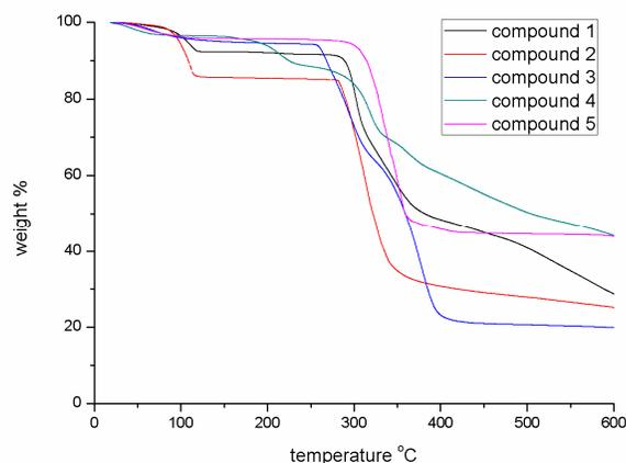
**Figure 6.** Thermogravimetric analysis plots of compounds **1-5**.
