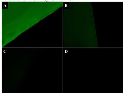
**Fig. 2** Protein (FITC-Fg) fouling test on hydrogels visualized under fluorescence microscope at the same excitation light intensity and exposure time. A) Dex-MA, B) CB-L-Dex, C) CB-H-Dex, and D) Control hydrogel surface with no protein contact.
