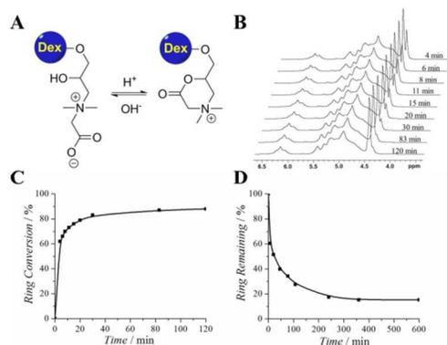
**Fig. 1** A) CB-H-Dex structural switch between zwitterionic form and cationic form. B) and C) the lactone ring formation of CB-H-Dex from zwitterionic form to its cationic ring form in TFA-d. D) the lactone ring open from cationic ring form to its zwitterionic form in D<sub>2</sub>O.
