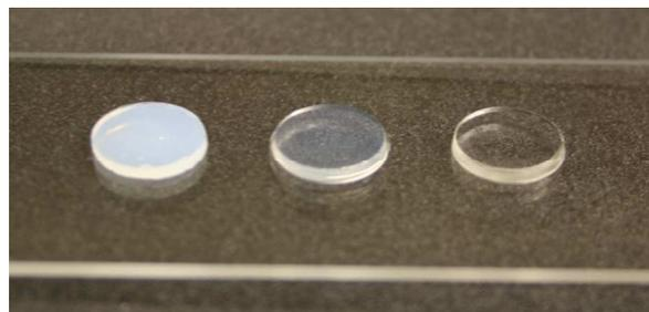
**Fig. 4** Digital image of dextran hydrogels. Left to right: Dex-MA, CB-L-Dex, CB-H-Dex.
