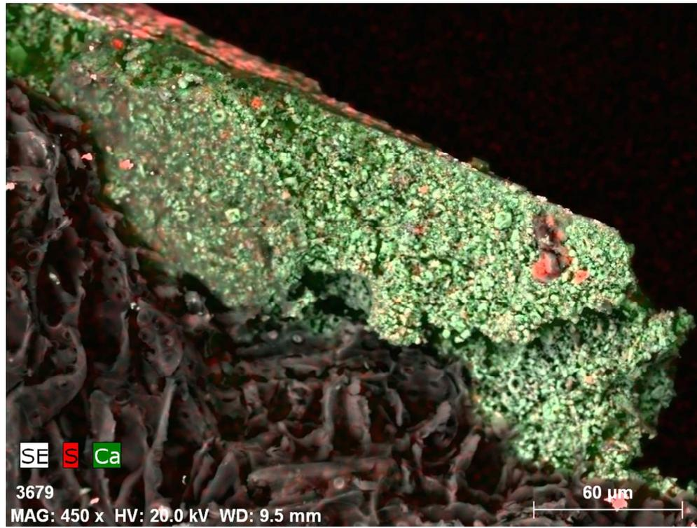
Fig 5a. Elemental analysis map by SEM-EDS detecting S and Ca in glue sizing of the painting Cristo e Pilatos (sample C-1) of group B.
