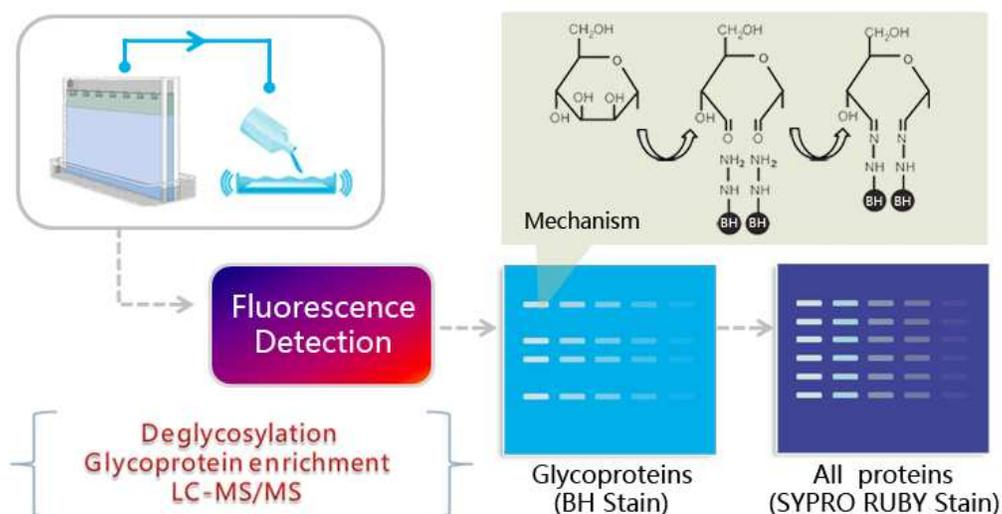
A sensitive, specific, economic and MS compatible staining method for gel-separated glycoproteins by using BH was described, meanwhile, the specificity of the newly developed stain for glycoproteins was demonstrated by 1-D and 2-D SDS-PAGE, deglycosylation, glycoprotein affinity enrichment and LC-MS/MS, respectively.
