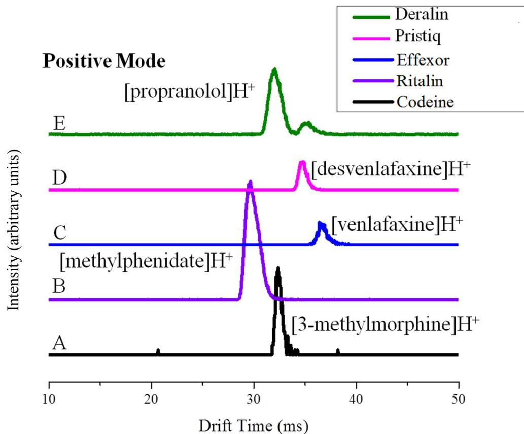
**Figure 3. Positive DESI-IMS-TOFMS Drug Standard Data.** The calculated  $K_o$  values for (A) Codeine ( $[3\text{-methylmorphine}]H^+$ ), (B) Ritalin ( $[methylphenidate]H^+$ ), (C) Effexor ( $[venlafaxine]H^+$ ), (D) Pristiq ( $[desvenlafaxine]H^+$ ) and (E) Deralin ( $[R/S\text{-propranolol}]H^+$ ) were 1.30, 1.46, 1.22, 1.17 and 1.26  $cm^2/Vs$ , respectively.
