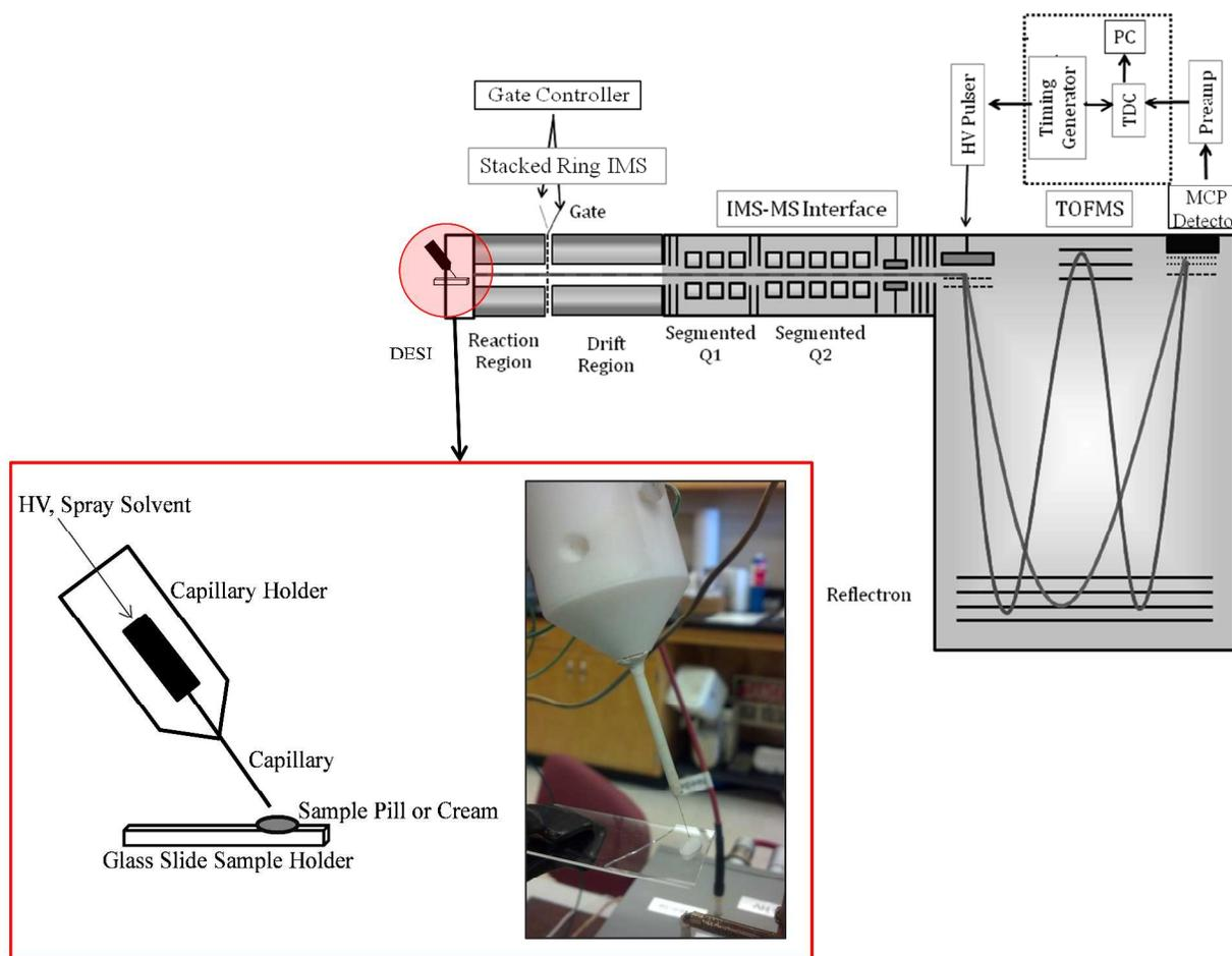
**Figure 1. IM-TOFMS Instrument Schematic.** Pictured from left to right is the DESI source, ion mobility spectrometer, IMS-MS interface (segmented Q1, segmented Q2 and lens region), TOF mass spectrometer and MCP detector. Insert shows DESI schematic and photograph of set up.
