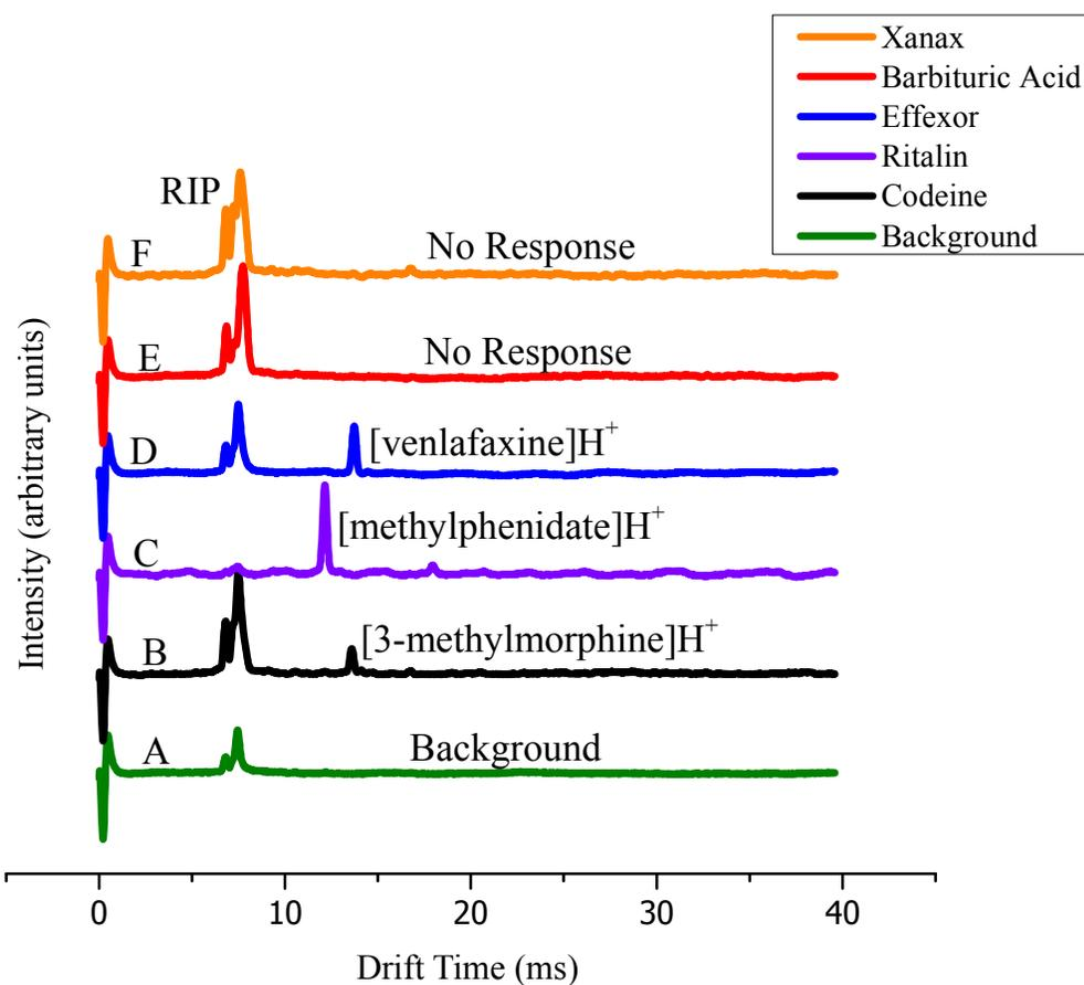
**Figure 2. Positive Mode Standalone DESI-IMS Drug Standard Data** The calculated  $K_o$  values for (B) Codeine ( $[3\text{-methylmorphine}]H^+$ ), (C) Ritalin ( $[methylphenidate]H^+$ ) and (D) Effexor ( $[venlafaxine]H^+$ ) were 1.27, 1.43 and 1.26  $cm^2/Vs$  ( $\pm 0.01cm^2/Vs$ ), respectively. (E) Barbituric acid and (F) Xanax were not detected in the positive mode.
