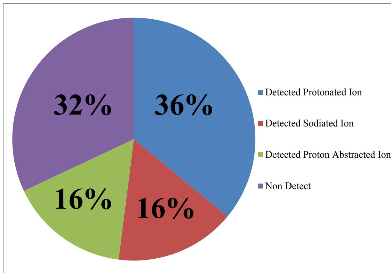
**Figure 7. Success Rates of DESI-IMS Method.** 68% of all samples analyzed (22 total) were successfully detected. 36% were detected in the positive mode as  $[M+H]^+$  ions, 16% were detected using reactive-DESI as  $[M+Na]^+$  ions and 16% were detected in the negative mode as  $[M-H]^-$  ions. 32% of the samples analyzed were not detected; however optimization of the current techniques could allow for a decreased non-detect percentage.
