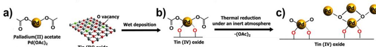
Scheme 1. Schematic illustration of synthesis of atomically dispersed tin (IV) oxide supported Pd catalyst: a) Wet deposition of Pd(OAc) 2 . b) Proposed structure of the (-SnO x )Pd(OAc) 2 surface complex, with the Pd center datively interacting with surface tin oxide. c) Thermal reduction of the resulting complex and proposed (-SnO x )Pd surface complex structure, with the Pd center datively interacting with the surface tin oxide.
