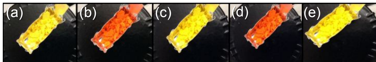
Figure 2. Photographs of a ground sample of yellow 1\cdot\text{PF}_6 in an aluminum weigh boat (a) pre- \text{CH}_3\text{CN} exposure and (b-d) for two \text{CH}_3\text{CN} sorption and desorption cycles. (b) Post \text{CH}_3\text{CN} sorption in the first cycle, (c) post \text{CH}_3\text{CN} desorption in the first cycle, (d) post \text{CH}_3\text{CN} sorption in the second cycle, (e) post \text{CH}_3\text{CN} desorption in the second cycle.
