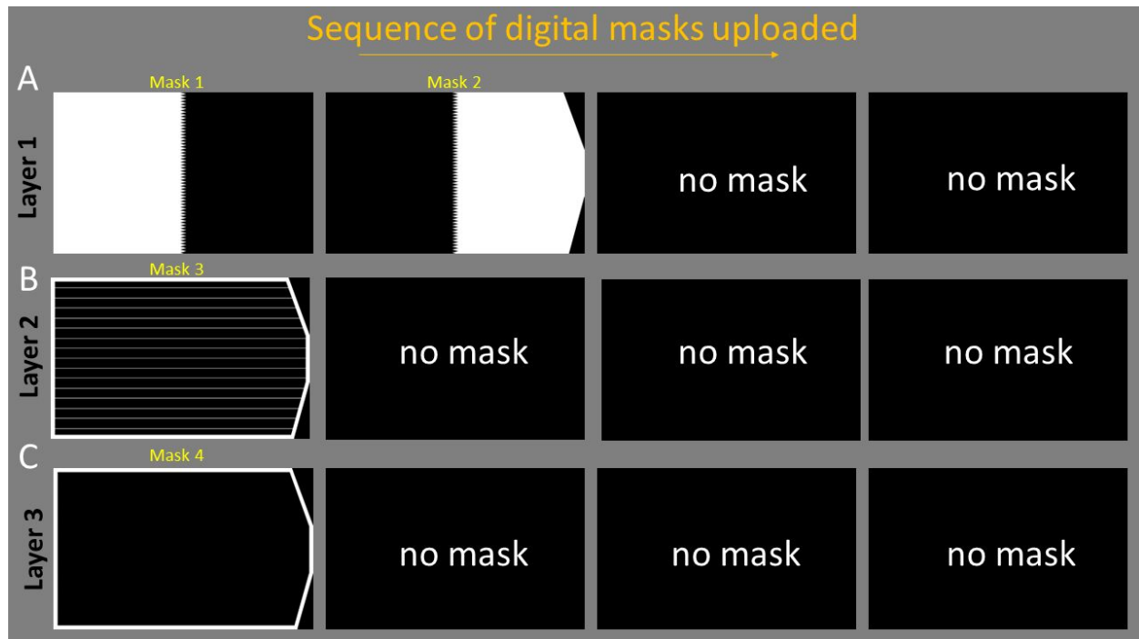
Supplementary Figure S1. Sequence of digital masks uploaded for the DLP-based 3D printing of PGSA-1STN scaffolds in a layer-by-layer fashion. (A) For layer 1, masks 1 and 2 were uploaded for the fabrication of the base layer. (B) For layer 2, mask 3 was uploaded for the fabrication of the microchannel walls plus outer walls. (C) For layer 3, mask 4 was uploaded for the fabrication of the outer walls.
