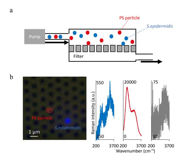
Figure 2. Capture and individual detection of microholes. (a) Schematic of microfiltration. (b) Fluorescence image and Raman spectra detected on the glass membrane filter. The fluorescence image was merged with the brightfield image. Blue Raman spectrum indicates Staphylococcus epidermidis, red Raman spectrum indicates PS particle, and gray Raman spectrum indicates filter hole.
