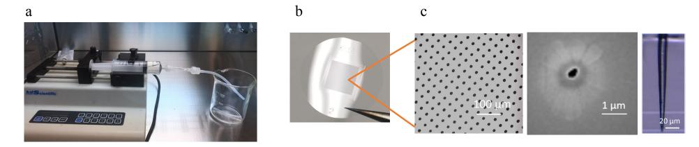
Figure 1. Microfiltration system for bacterial cells. (a) Photograph of the filtration device. (b) Photograph of 9.5 mm filter. (c) Microscopic image of the filter. Planar view of multiple and single hole followed by cross section of single hole.
