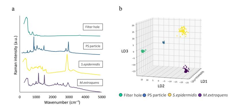
Figure 4. Discriminant analysis of microfiltration. (a) Pattern of Raman spectra detected on the glass membrane filter. (b) LDA results for Raman spectra detected on the glass membrane filter.
