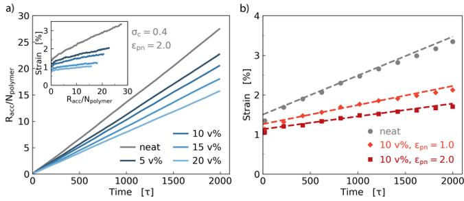
Fig. 6 a) Normalized  $R_{acc}$ , as a function of time, for different NP loadings at  $T = 0.40$  and  $\sigma_c = 0.4$ . The inset shows the corresponding strain versus  $R_{acc}/N_{polymer}$  curves. b) Predicted strain-time responses (dashed lines) of three systems at  $T = 0.40$ ; dots are the measured strain. These simulations use neat polymers or  $r = 3\sigma$  PNCs.
