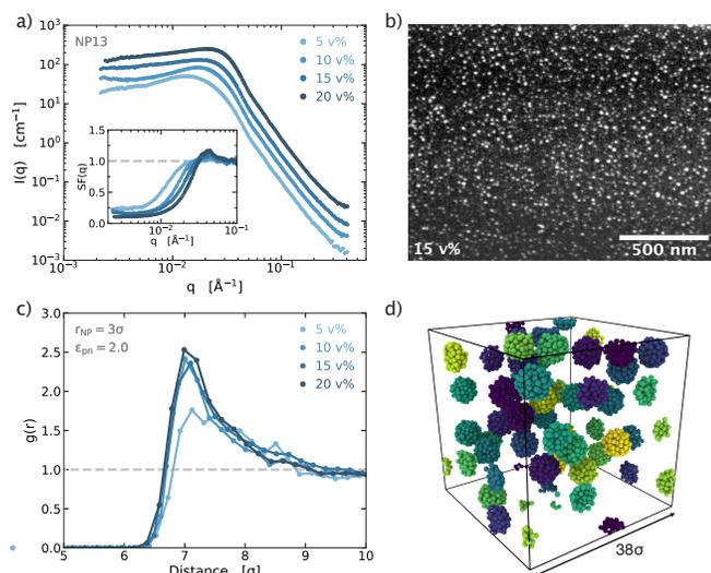
Fig. 1 a) SAXS measurements of NP13 composites showing excellent NP dispersion with an inset showing the NP structure factor. b) Representative SEM image of the 15 vol% NP13 PNCs. c) Pair distribution functions of NPs in simulated PNCs with small attractive NPs ( $r = 3\sigma$ ) showing good dispersion. d) Visualization of the NP distribution in the simulated PNCs with small attractive NPs (10 vol% NP). NPs are colored to ease differentiation.
