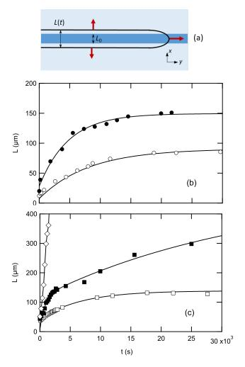
**Fig.** 5 Width L of the debonded strip as a function of time  $(L_0=9\,\mu\mathrm{m})$ . (a) schematic of delamination width L(t) along x direction from an interface defect width  $L_0$  with  $L(t=0)\approx L_0$ ; (b) film thickness  $h=(\circ)$  770 and  $(\bullet)$  1130 nm with a grafting density of 0.6 nm $^{-2}$ ; (c) film thickness  $h=(\Box)$  480, ( $\blacksquare$ ) 700 and  $(\diamondsuit)$  1060 nm with a grafting density of 0.2 nm $^{-2}$ . Solid lines are guides for the eye.
