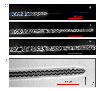
**Fig. 2** Phone cord debonding mechanisms from a defect line  $L_0=9~\mu\mathrm{m}$  in width ( $h=700~\mathrm{nm}$ , grafting density of 0.6  $\mathrm{nm}^{-2}$ , swelling ratio S=2.7). (a) images of the swollen film taken (i) 360 , (ii) 420 and (iii) 620 s after exposure to humid air. The blue areas and the dotted blue line indicates the line defect width  $L_0$  and orientation, respectively. (b) microscopic image of the dried debonded hydrogel with the tip of the debonded area.
