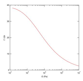
**Fig. 11** Non dimensional strain energy release rate  $\Gamma/Gh$  for the delamination of a film with dry thickness h as a function of the shear modulus G of the drained hydrogel network ( $\chi = 0.57$ ,  $kT/v = 1.37 \, 10^8 \, \mathrm{Pa}$ ).
