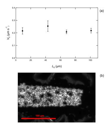
**Fig. 4** Debonding from defect strips with widths  $L_0$  ranging from 9 to 100  $\mu$ m (h=680 nm, grafting density of 0.6 nm $^{-2}$ , swelling ratio S=3.8). (a) initial debonding velocity  $V_0$  as a function of  $L_0$ . (b) image of the debonded line for  $L_0=100~\mu$ m showing extensive folding of the debonded film.
