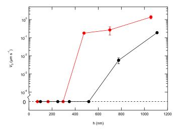
Fig. 8 Debonding velocity  $V_0$  as a function of dry film thickness h for films with a grafting density of ( $\bullet$ ) 0.2 nm<sup>-2</sup> and ( $\bullet$ ) 0.6 nm<sup>-2</sup>.
