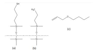
**Fig. 1** Silicon wafer grafted with (a) (3-mercaptopropyl)trimethoxysilane and (b) propylsilane. (c) Allyl butyl ether used to passivate the grafted thiol groups.
