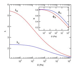
**Fig. 10** Theoretical swelling ratios  $\lambda$  calculated for the bonded (red,  $\lambda_B$ , Eq. (3)) and the plane strain delaminated parts of the film (blue,  $\lambda_A$ , Eq. (4)) as a function of the shear modulus G of the drained network ( $\chi=0.57, kT/\nu=1.38\,10^8\,\mathrm{Pa}$ ). Inset: corresponding volume fractions  $\Phi_A$  and  $\Phi_B$  of water within the swollen network.
