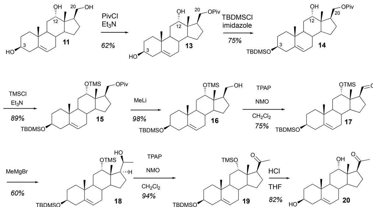
Scheme 2. Synthesis of 12 $\alpha$ -hydroxypregnenolone (**20**) from triol **11**.
