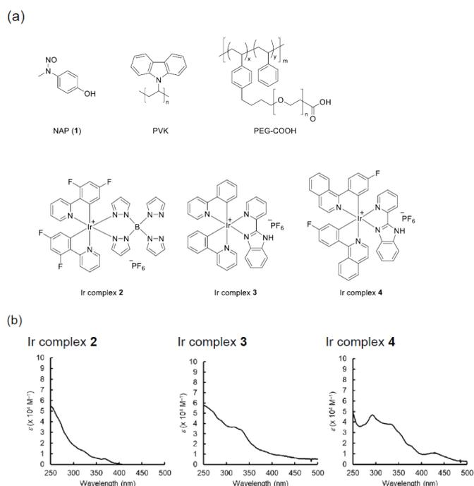
Figure 1. (a) Structures of **1–4**, PVK, and PEG-COOH. (b) Measurements of absorption spectra of Ir complexes **2–4**. Absorption spectra of a solution of **2–4** (10  $\mu\text{M}$ ) in THF were recorded.
