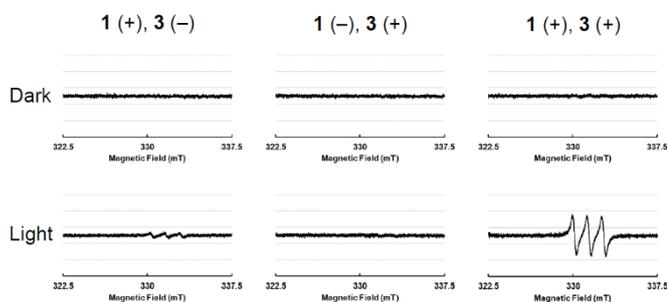
Figure 4. ESR measurements. A suspension containing P-dots doped with **1** and **3**, FeSO<sub>4</sub>·7H<sub>2</sub>O (1.5 mM), and *N*-methylglucamine dithiocarbamate (6 mM) in HEPES was irradiated at 430–460 nm (12 mW cm<sup>-2</sup> for 10 min).
