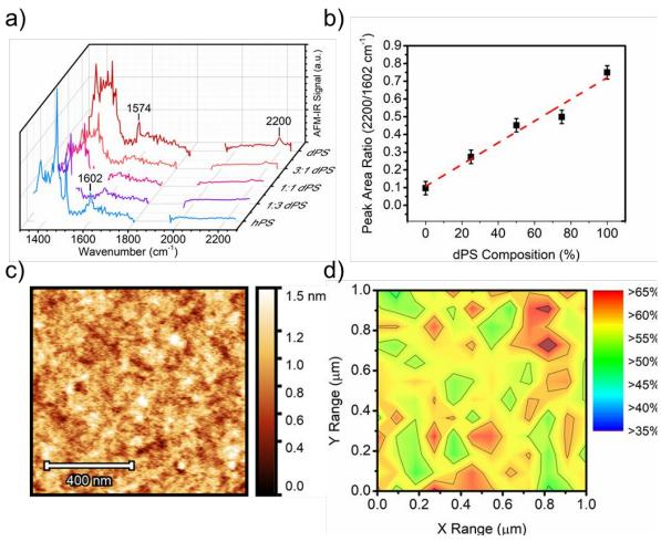
**Figure 4.** Using deuterium to distinguish the isotope polymer blends. (a) Broadband AFM-IR spectrum acquired from dPS:hPS films of different blend ratios. (b) Calibration curve generated from the broadband spectra collected in (a). (c) height image of 1:1 (v/v) dPS:hPS blend. (d) Composition map of area highlighted in **Figure 4c** where percentage values indicate dPS fraction.
