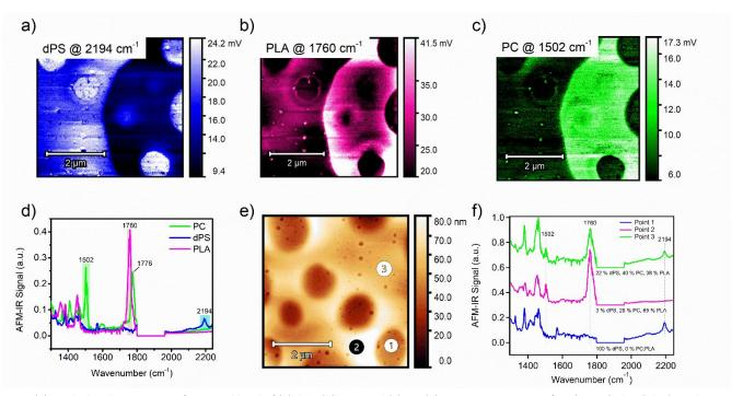
Figure 3. (a) Single-band IR imaging of ternary blend of (a) dPS, (b) PLA, and (c) PC. (d) AFM-IR spectrums of PC (green), dPS (blue), and PLA (magenta) with highlighted peaks chosen for single-band AFM-IR scans. (e) Height image of an equal-weighted ternary blend composed of dPS:PLA:PC. (f) AFM-IR spectra of points 1, 2, and 3 indicated in Figure 3e, with included composition values for dPS, PLA, and PC for those points.
