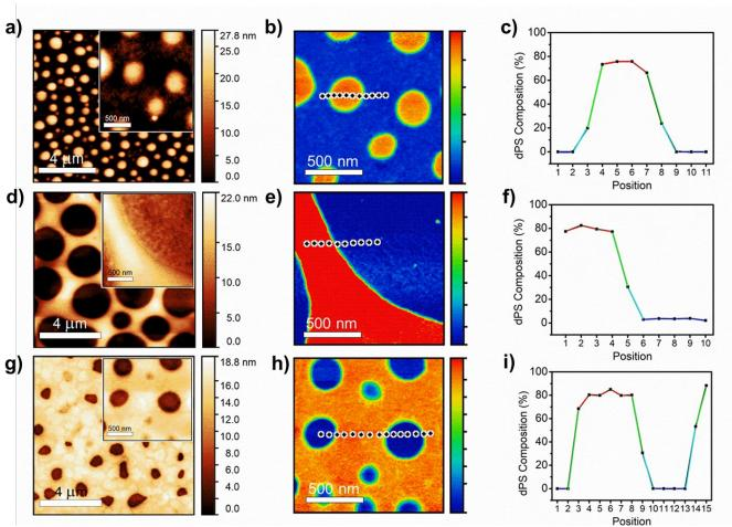
Figure 2. Detailed height image, infrared image, and composition curve of (a-c) dPS:P3HT (1:3), (d-f) dPS:P3HT (1:1), and (g-i) dPS:P3HT (3:1).
