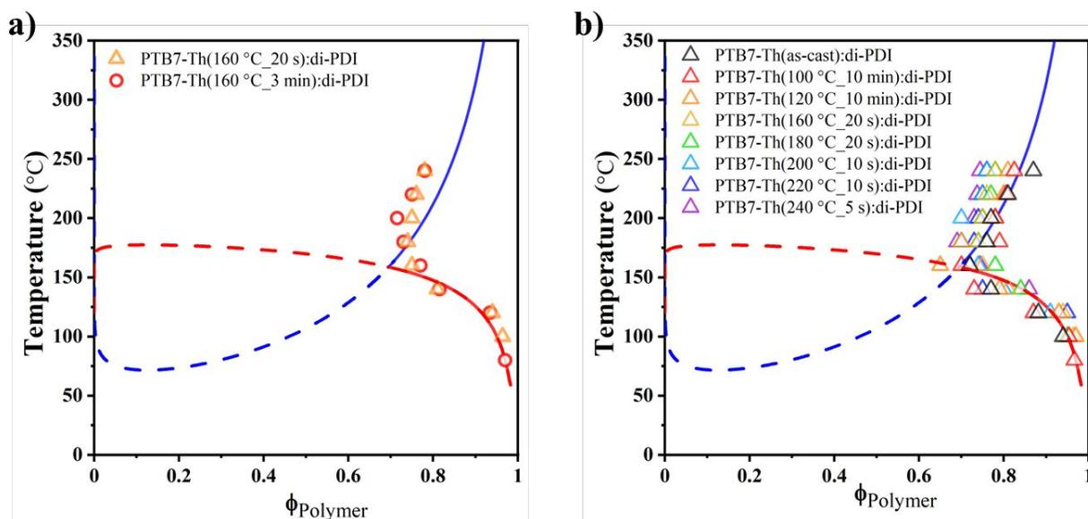
**Figure 3.** a) Comparison between the phase diagram from pre-annealing PTB7-Th layers at 160 °C for different time. The consistency suggests that 20 s pre-annealing is enough for structural recovery at 160 °C. b)  $T - \phi$  phase diagram for PTB7-Th:di-PDI with PTB7-Th thin film pre-annealed at different temperatures before making bilayers to allow polymer chains relax. The dashed/solid lines represent the UCST or LCST Flory-Huggins fits for as-cast films as guides to the eye.
