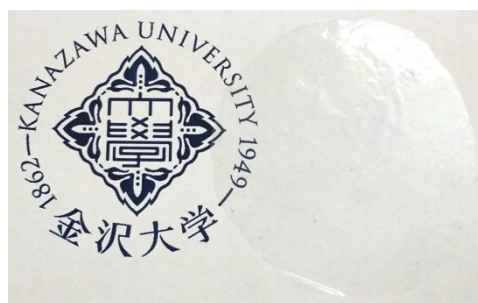
Figure 5. Photograph of cellulose dimethylphenylsilyl ether films (DS = 2.57) obtained via Scheme 2 cast from dichloromethane solution.
