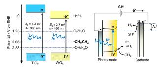
Figure 2. (a) Energy band diagram of  $TiO_2$  and  $WO_3$ . (b) PEC process using photoanode and cathode under applied bias ( $\Delta E$ ).
