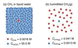
Figure 3. (a) Molar concentrations of (a) dissolved  $CH_4$  and  $H_2O$  in liquid water, and (b) gaseous  $CH_4$  and water vapor in humidified condition at 25°C.
