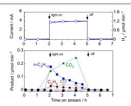
Figure 7. PEC activation of  $C_2H_6$  using  $WO_3$  photoanode under visible-light irradiation (6.8 mW cm<sup>-2</sup> at 453 nm) at 1.2 V; (a) the overall current and  $H_2$  evolution rate on the cathode side, and (b) the rates of product formation on the photoanode side.
