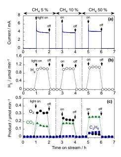
Figure 5. Effect of  $CH_4$  concentration on the PEC reactions over the  $WO_3$  photoanode:(a) the overall current at 1.2 V, (b) the rate of  $H_2$  evolution on the cathode side, and (c) the rate of products formation on the photoanode side under visible-light irradiation (6.8 mW cm<sup>-2</sup> at 453 nm).
