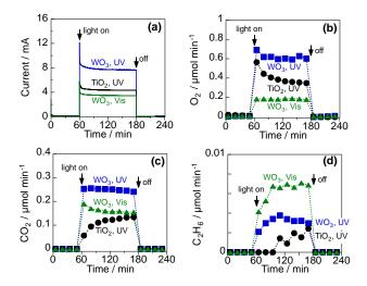
Figure 4. PEC activation of 10 vol%  $CH_4$  using  $WO_3$  and  $TiO_2$  photoanodes under UV light (6.5 mW cm<sup>-2</sup> at 365 nm) and visible light (6.8 mW cm<sup>-2</sup> at 453 nm): (a) the overall current at 1.2 V, (b) the rate of  $O_2$  evolution, (c) the rate of  $CO_2$  formation, and (d) the rate of  $CO_2$  formation on the photoanode side.
