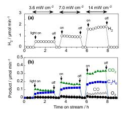
Figure 6. Effect of light intensity on the activation of humidified  $CH_4$  using the  $WO_3$  photoanode under 453-nm irradiation at 1.2 V; (a) the  $H_2$  evolution rate on the cathode side and (c) the rates of product formation on the photoanode side .
