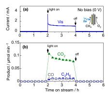
Figure 9. PEC oxidation of  $CH_4$  by the PEM-PEC reactor using the  $WO_3$  photoanode and Pt/carbon catalyst: (a) the overall current at zero bias, and (b) the rate of products formation on the photoanode side under 453-nm light irradiation (6.8 mW cm<sup>-2</sup>).
