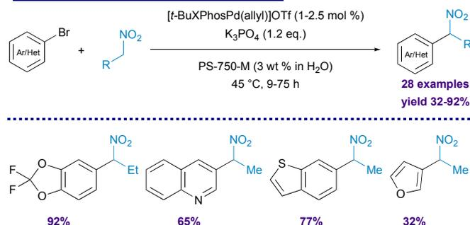
Scheme 1: First application of PS-750-M technology in transition-metal catalyzed sp<sup>2</sup>-sp<sup>3</sup> cross-couplings.
