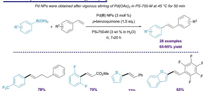
Scheme 9: Ligand-free ultrasmall Pd(0) nanoparticles for Mizoroki-Heck-type couplings.
