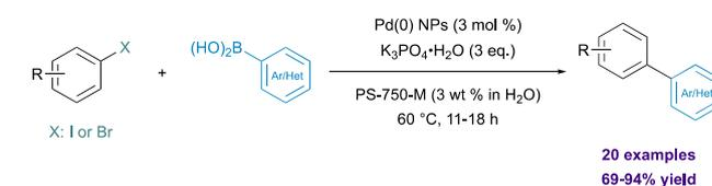
Scheme 10. Ligand-free Pd(0) nanoparticles for Suzuki-Miyaura couplings.
