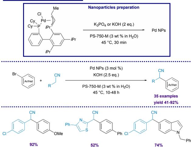
Scheme 2: Pd nanoparticles-catalyzed  $\alpha$ -arylation of nitriles.
