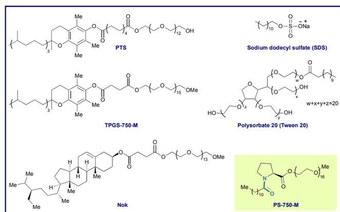
Figure 1. Examples of different state-of-the-art surfactants.
