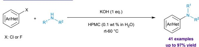
Scheme 16: Nucleophilic aromatic substitution in water using HPMC as additive.
