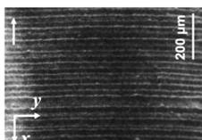
Figure 2: Representative image of polystyrene (PS) particle bands printed on NCAMs. The printing was done at an applied electric field strength of  $-35 \text{ V}/\text{cm}$  and a volumetric flow rate of  $5 \mu\text{L}/\text{min}$ . The pressure difference driving the Poiseuille flow and the electric field are in opposite directions. Nominal diameter of PS particles was  $490 \text{ nm}$ . NCAMs present a pore diameter of  $220 \text{ nm}$  to permit excess fluid drainage.
