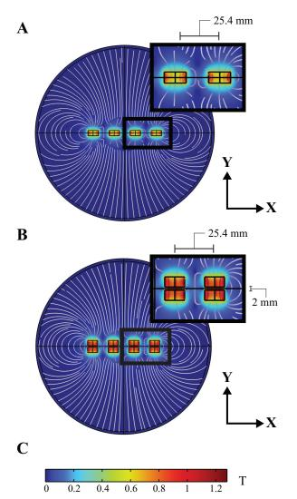
Fig. 4 COMSOL simulations of (A) one row and (B) two rows of neodymium magnets in the  $2 \, mm$  spacing case with the magnetic field lines in white and xy reference frames. (C) shows the magnetic flux density norm that applies to (A) and (B).
