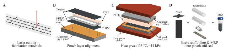
Fig. 3 Fabrication of MRJ beams process. (A) Materials are laser cut to size. (B) Textile, TPU, and PTFE are aligned to create the pouch of the beam. (C) Pouch elements are bonded on the heat press for 4 min. (D) Scaffolding material and 1 ml of magnetorheological fluid (MRF) are inserted into the pouch, which is then hand-sealed.
