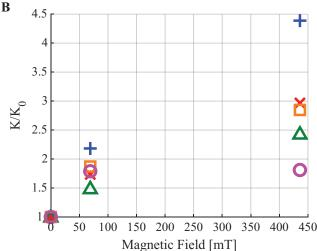
Fig. 9 Stiffness vs. Magnetic Field for various MRJ beam scaffolding designs. The stiffness of each MRJ beam is normalized by its initial stiffness at 0 mT. (A) Results due to the single row of magnets, i.e. MR effect. (B) Results due to the double row of magnets, i.e. MR and clutch effect.
