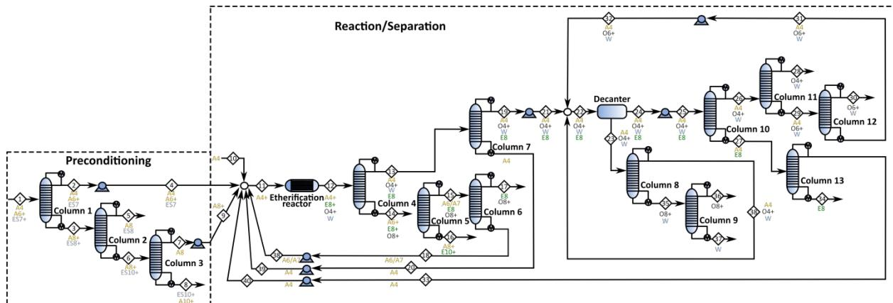
**Figure 7.** Layout for the etherification area. Chemical species in the figure are labelled using the following convention: a letter indicates the functional group (A: alcohols, O: olefins, E: ethers, UA: Unidentified components), and a numerical character the carbon length.
