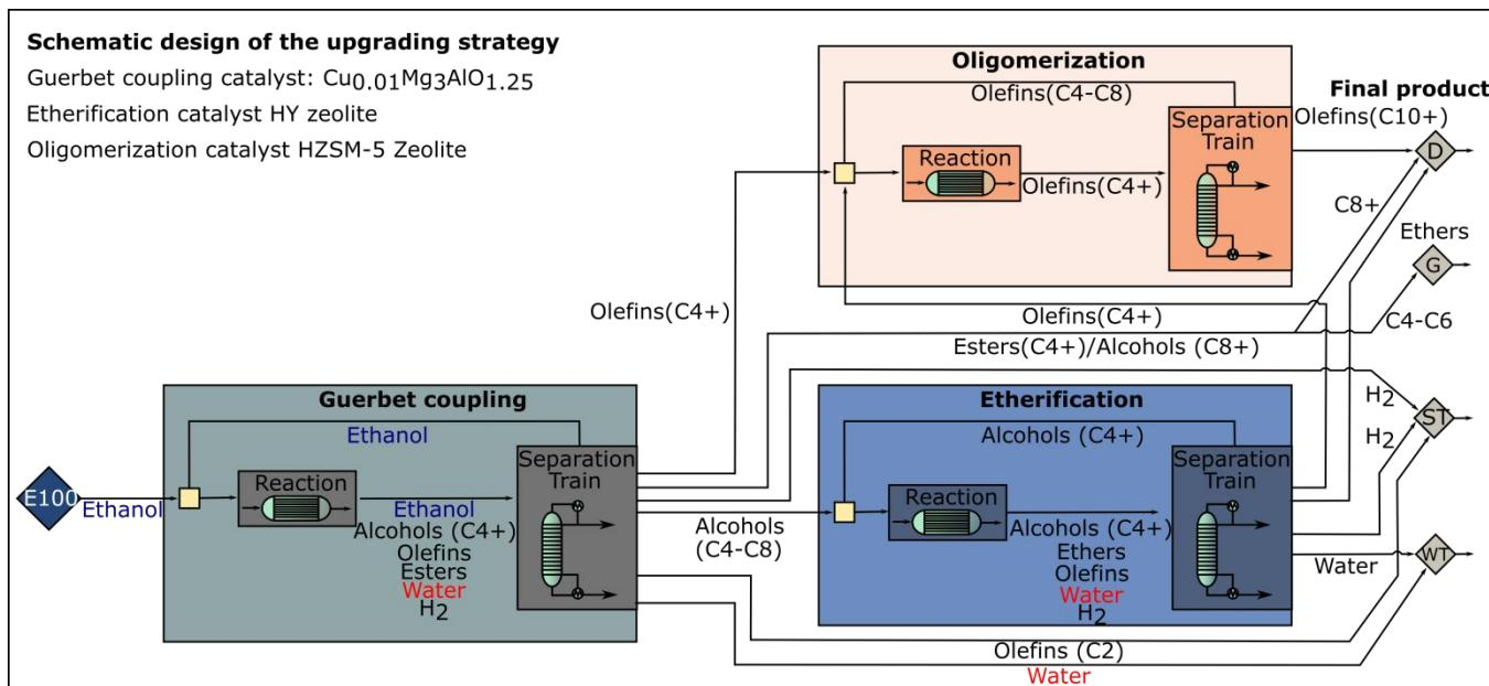
**Figure 1.** Schematic representation of an ethanol upgrading biorefinery based on Guerbet coupling, etherification, and olefin oligomerization. D: Diesel, G: Gasoline, ST: Steam, WT: Waste water.
