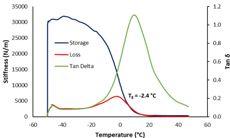
**Figure 8.** Thermomechanical analysis (TMA) of **C1** (-S-H:-O-CN =1)
