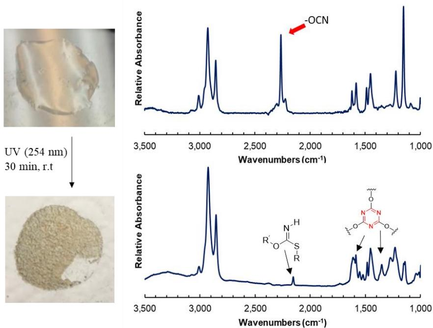
**Figure 5.** Digital images of an uncured mixture of **1** and **3** (top left,  $-\text{SH}:-\text{OCN}$  ratio of 1) and cross-linked network (bottom left, 254 nm UV irradiation, 30 min). FTIR spectra of the uncured mixture (top right) and cross-linked network (bottom right).
