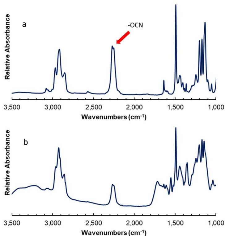
**Figure 6.** FTIR spectra showing partial cyclotrimerization of the cyanate ester in 4,4'-(propane-2,2-diyl)bis(2-allyl-1-cyanatobenzene) (**4**) upon blending with **3** and UV light exposure. a) Uncured mixture and b) partially cured mixture after exposure to UV radiation.
