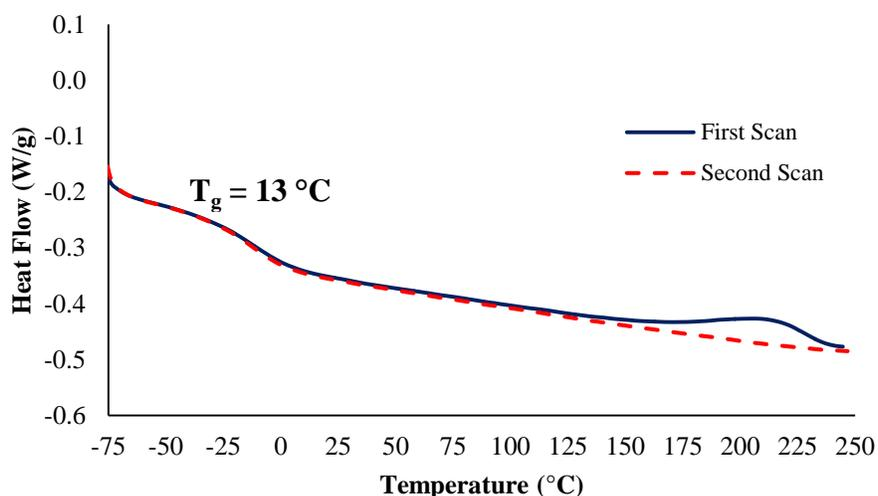
**Figure 7.** DSC of a cross-linked cardanol cyanate ester trithiol blend (**C1**) with an -S-H/-O-CN ratio of one.
