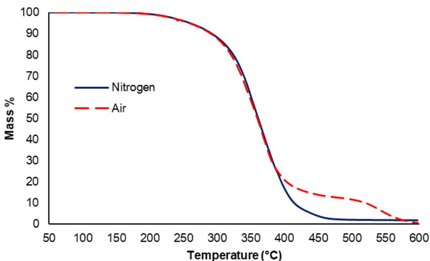
**Figure 9.** Thermogravimetric Analysis (TGA) of **C1** (-S-H:O-CN = 1)
