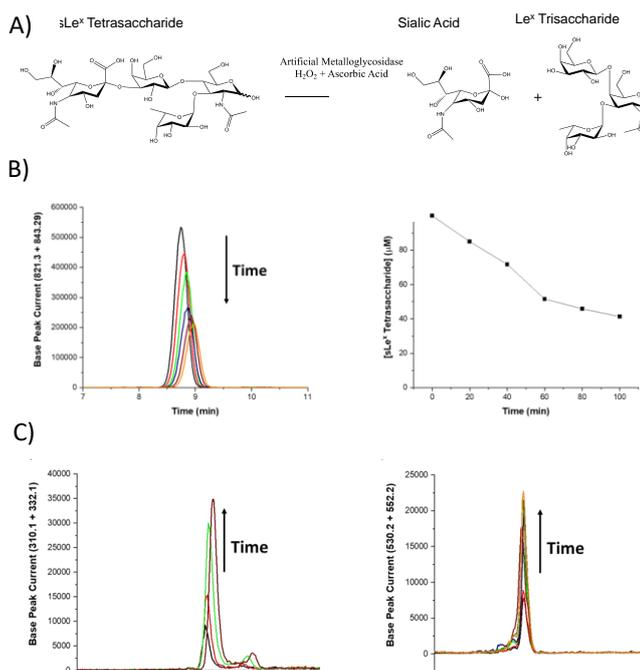
**Figure 2.** Metalloprotein reaction scheme and base peak current (BPC) chromatograms. A) Proposed reaction mechanism. B) Reactant BPC chromatogram (left) and reaction progress (right) for sLe<sup>x</sup> substrate for the Cu-ATCUN-tOL peptide reaction, C) BPC chromatogram for sialic acid (left) and Le<sup>x</sup> trisaccharide (right) products.
