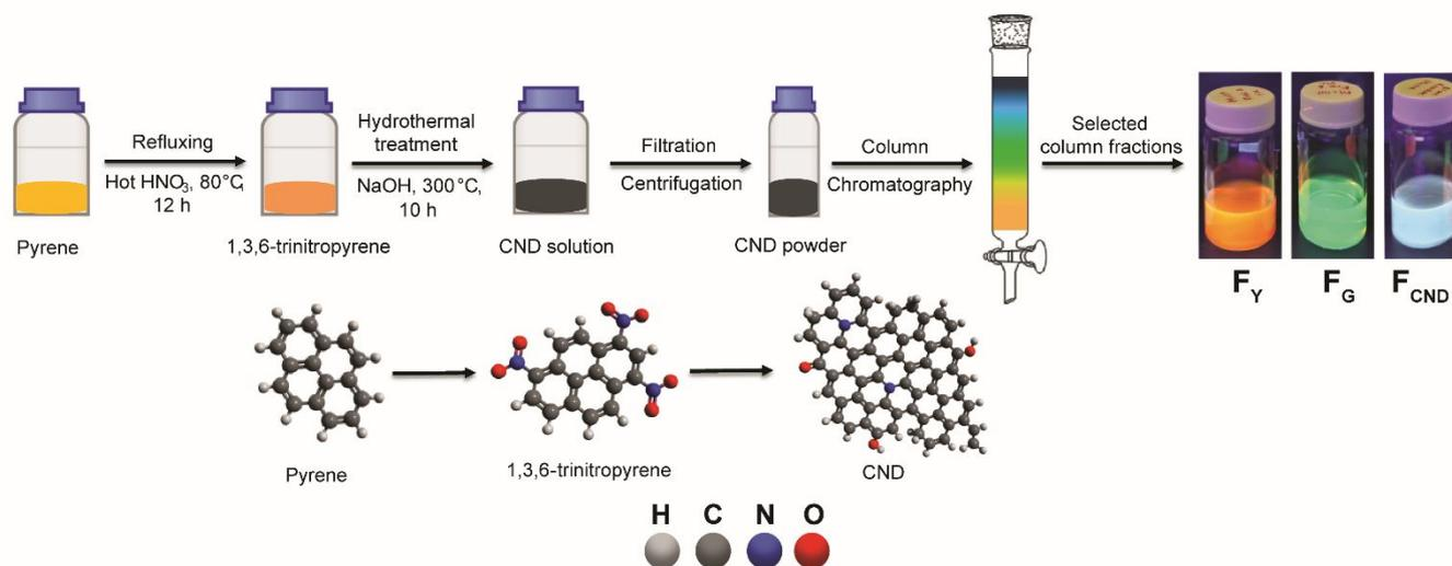
Scheme 1. Procedures to synthesize CNDs and separate fractions through column chromatography. At the bottom, it presents the hypothetical scheme of the synthesis starting from pyrene, to TNP, and to CND.
