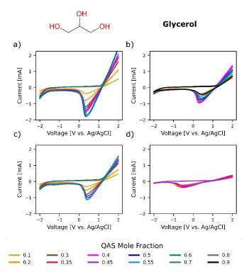
**Figure 14** Cyclic voltammograms of Glycerol-based DES as a function of QAS mole fraction. For all measurement, the potential was varied from -2V and 2V with a scan rate of 100 mV/s and a total of 4 cycles per sample to ensure equilibration. The position of the feature on the backward scan seems to be dependent on the halide anion of the QAS component. a) Choline Chloride, b) Acetylcholine Chloride, c) Tetraethylammonium Chloride, d) Tetrapropylammonium Bromide
