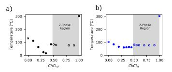
Figure 8 Phase diagrams for urea (a) and N,N'-dimethylurea (b). The filled circular markers indicate measurements obtained using the PhasIR system. The x-shaped markers indicate literature values for the pure components.
