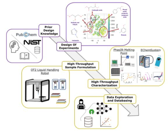
Figure 1 Schema for the high-throughput protocol for DES selection, processing, and characterization. The purple boxes represent the initial data-driven candidate selection for both DES components (QASs & HBDs), whereas the gold boxes represent the automatic sample formulation, processing, characterization, and final data analysis of the prepared samples.
