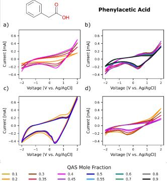
**Figure 11** Cyclic voltammograms of phenylacetic acid-based DES as a function of QAS mole fraction. For all measurement, the potential was varied from -2V and 2V with a scan rate of  $100 \ mV/s$  and a total of 4 cycles per sample to ensure equilibration. a) Choline Chloride, b) Acetylcholine Chloride, c) Tetraethylammonium Chloride, d) Tetrapropylammonium Bromide
