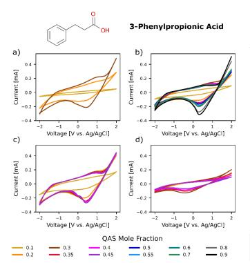
**Figure 12** Cyclic voltammograms of 3-phenylpropionic acid-based DES as a function of QAS mole fraction. For all measurement, the potential was varied from -2V and 2V with a scan rate of  $100 \ mV/s$  and a total of 4 cycles per sample to ensure equilibration. a) Choline Chloride, b) Acetylcholine Chloride, c) Tetraethylammonium Chloride, d) Tetrapropylammonium Bromide
