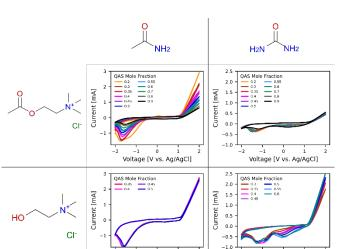
**Figure 13** Comparison between the cyclic voltammograms of Acetamide (Left) and Urea (Right) in their combinations with Acetylcholine Chloride (Top) and Choline Chloride (Bottom). The two HBD have similar molecular structure and it is possible to show parallel between the CV features in the backward scan. The two QAS both have Chlorine as their halide anion and show similarities in their voltammograms
