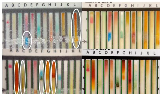
Figure 4. Wax-printed and air-gap pharmaceutical screening PADs. Left panels show wax-printed 12-lane PADs for ciprofloxacin (top) and isoniazid (bottom) with expected color changes circled. Right panels show air-gap PADs for ciprofloxacin (top) and isoniazid (bottom). Images of all 25 air-gap PADs read by the human evaluators can be found in the supplemental information.
