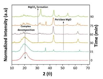
**Figure 7.** Depicting the morphological changes of the MgO catalyst at different reaction times. XRD data of the recovered catalyst at the corresponding reaction time.
