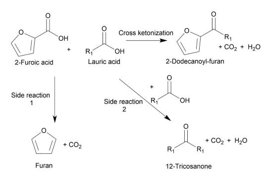
**Figure 2**. Scheme for the overall ketonization reaction between 2-furoic acid and lauric acid ( $R_1=C_{11}H_{23}$ ). The side reactions 1 and 2 are the decarboxylation of 2-furoic acid to furan and the lauric acid self-ketonization to 12-tricosanone.
