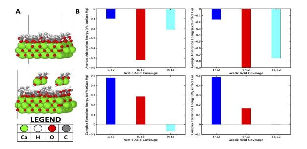
**Figure 8** (a) Image showing the simulation for the 11/12 ML model of acetic acid adsorbed on CaO (001) surface and the corresponding complex formation (top and bottom images, respectively). (b) The top row shows the average adsorption energy as a function of coverage of acetic acid, and the bottom row shows the corresponding complex formation energy for a given coverage.
