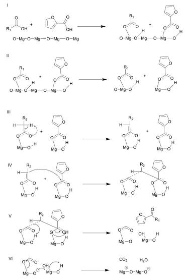
**Figure 10**. Proposed reaction mechanism for cross ketonization of lauric and 2-furoic acid based on computational and experimental evidence presented in this work
