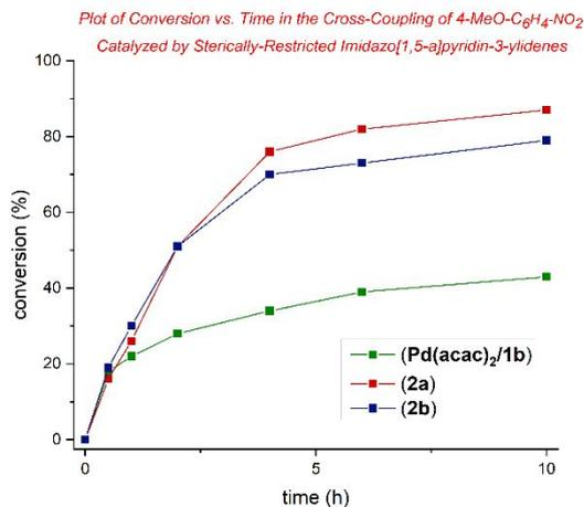
**Figure 3.** Kinetic profile of the Suzuki-Miyaura cross-coupling of 4-MeO-C<sub>6</sub>H<sub>4</sub>-NO<sub>2</sub> with phenylboronic acid catalyzed by Pd(acac)<sub>2</sub>/1b, 2a and 2b at 130 °C.
