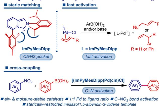
**Figure 1.** (A) Electronic and structural remodelling of NHC ligands. (B) State-of-the art Pd(II) precatalysts in cross-coupling reactions. (C) Pd(II)-ImPy and steric-matching of [(ImPyMesDipp)Pd(cin)Cl] as air-stable, fast-activating, sterically-restricted Pd(II)-NHC precatalysts.
