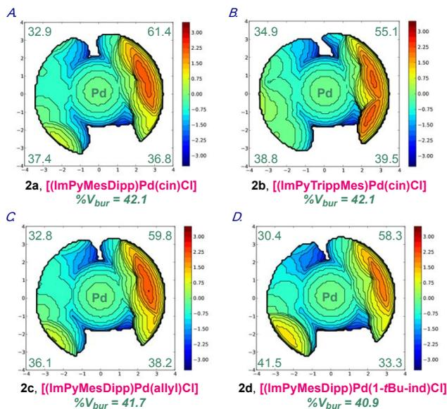
**Figure 5.** Topographical steric maps of [(ImPyMesDipp)Pd(cin)Cl] (**2a**) (A), [(ImPyTrippMes)Pd(cin)Cl] (**2b**) (B), [(ImPyMesDipp)Pd(allyl)Cl] (**2c**) (C), [(ImPyMesDipp)Pd(1-*t*Bu-ind)Cl] (**2d**) (D) showing %  $V_{bur}$  per quadrant.
